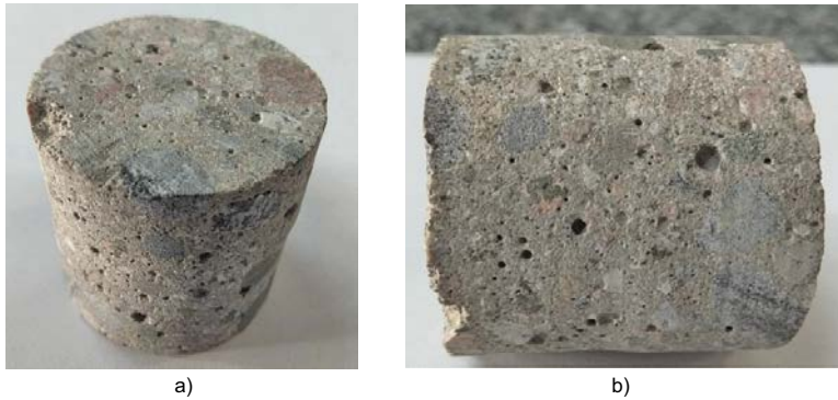
Figure 5-30. Elevation (a) and lateral (b) views of BMA-B5 sample for gas permeability tests.
