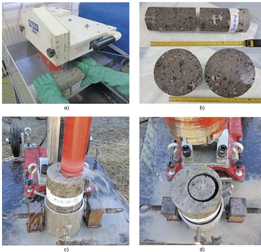
Figure 2-5. Sample preparation: cutting ETAPP core into two pieces using a diamond disk (a–b); drilling of the ETAPP sub-cores by using a core drill bit (c–d).
