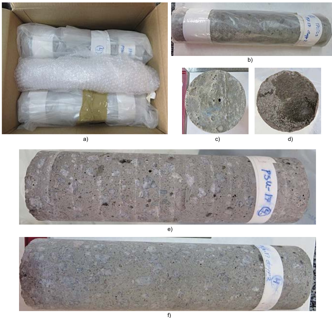
Figure 2-1. ETAPP concrete samples in the original packing at the reception (a–b); appearance of the upper (c) and lower (d) sides of one ETAPP1 core; lateral view of ETAPP1 (e) and ETAPP2 (f) cylindrical samples.
