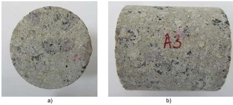
Figure 5-16. Front (a) and lateral (b) views of TAS05_09-A3 sample for gas permeability tests.
