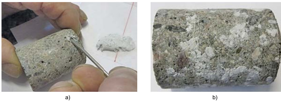
Figure 5-26. Application of the filler in the surface cavities of the concrete sample (a) and final appearance after filling the cavities (b).
