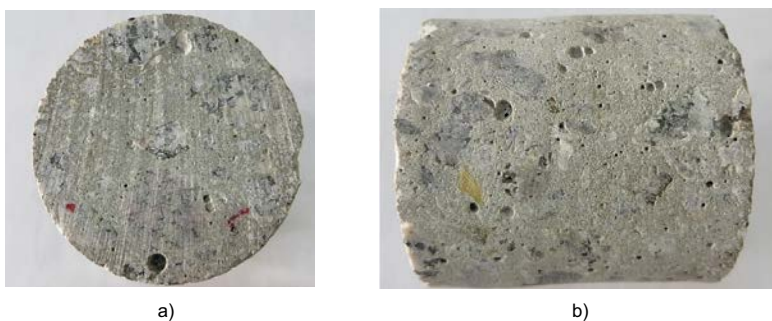
Figure 5-7. Front (a) and lateral (b) views of ETAPP1-6-I-2 sample for gas permeability tests.
