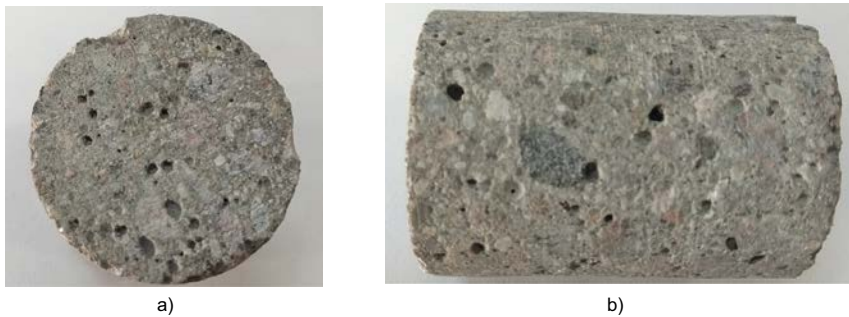
Figure 5-24. Front (a) and lateral (b) views of OPC-P5 sample for gas permeability tests.
