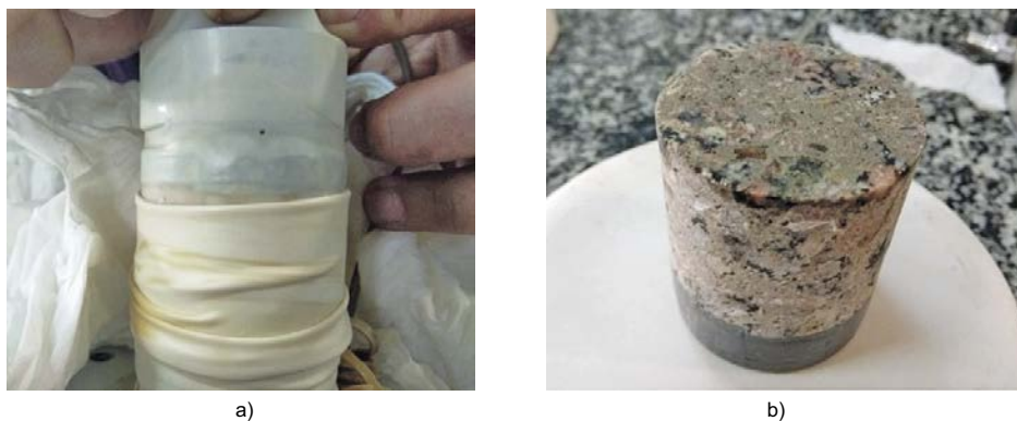
Figure 5-23. Piercing of membranes (a) and sample wetted at the upper end after failure (b).
