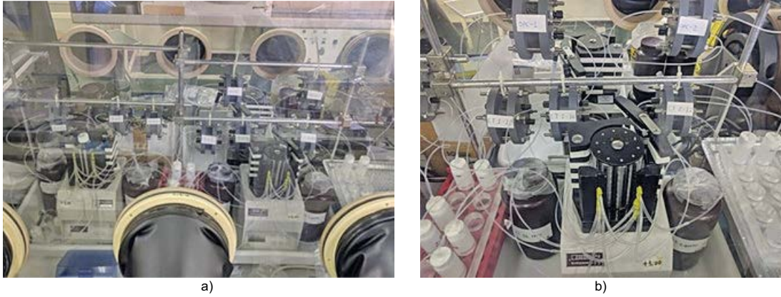
Figure 7-2. Experimental setup of diffusion cells into the glove box (a); detail of the setup with the inlet and outlet reservoirs at both sides of the diffusion cell (b).
