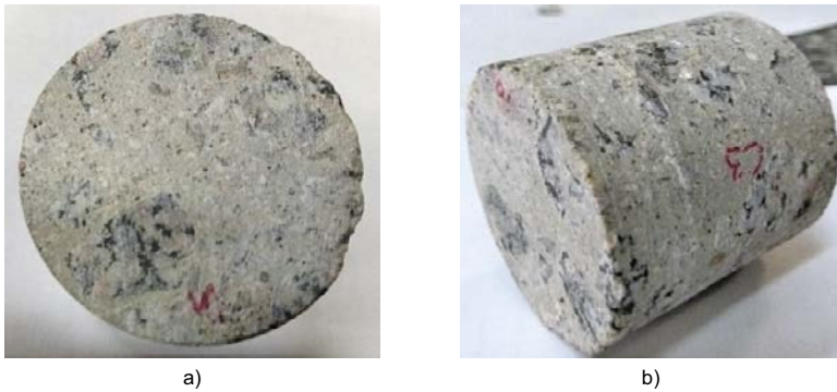
Figure 5-20. Front (a) and lateral (b) views of TAS05_09-C3 sample for gas permeability tests.
