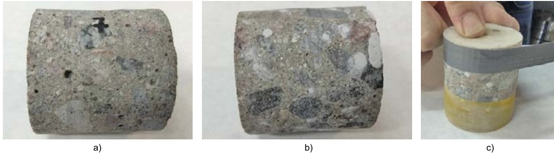
Figure 5-34. Lateral views of BMA-B7 sample (a–b) for gas permeability tests and preparation of the sample before wrapping (c).
