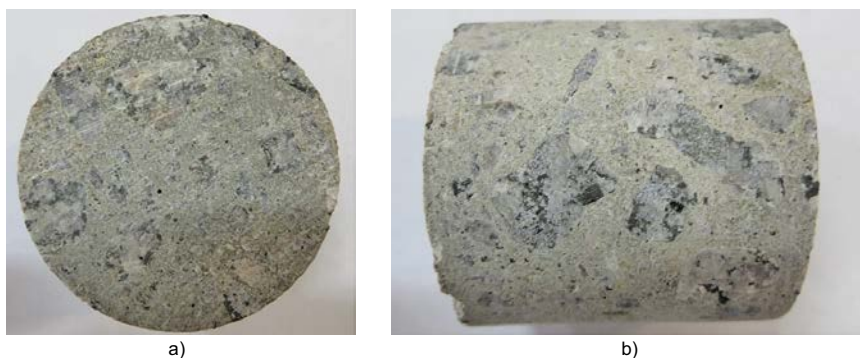
Figure 5-13. Front (a) and lateral (b) views of ETAPP2-2-I-4 sample for gas permeability tests.
