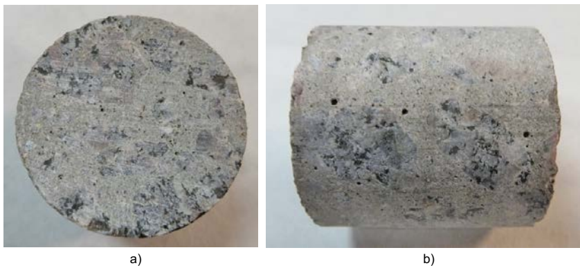
Figure 5-10. Front (a) and lateral (b) views of ETAPP2-2-I-2 sample for gas permeability tests.
