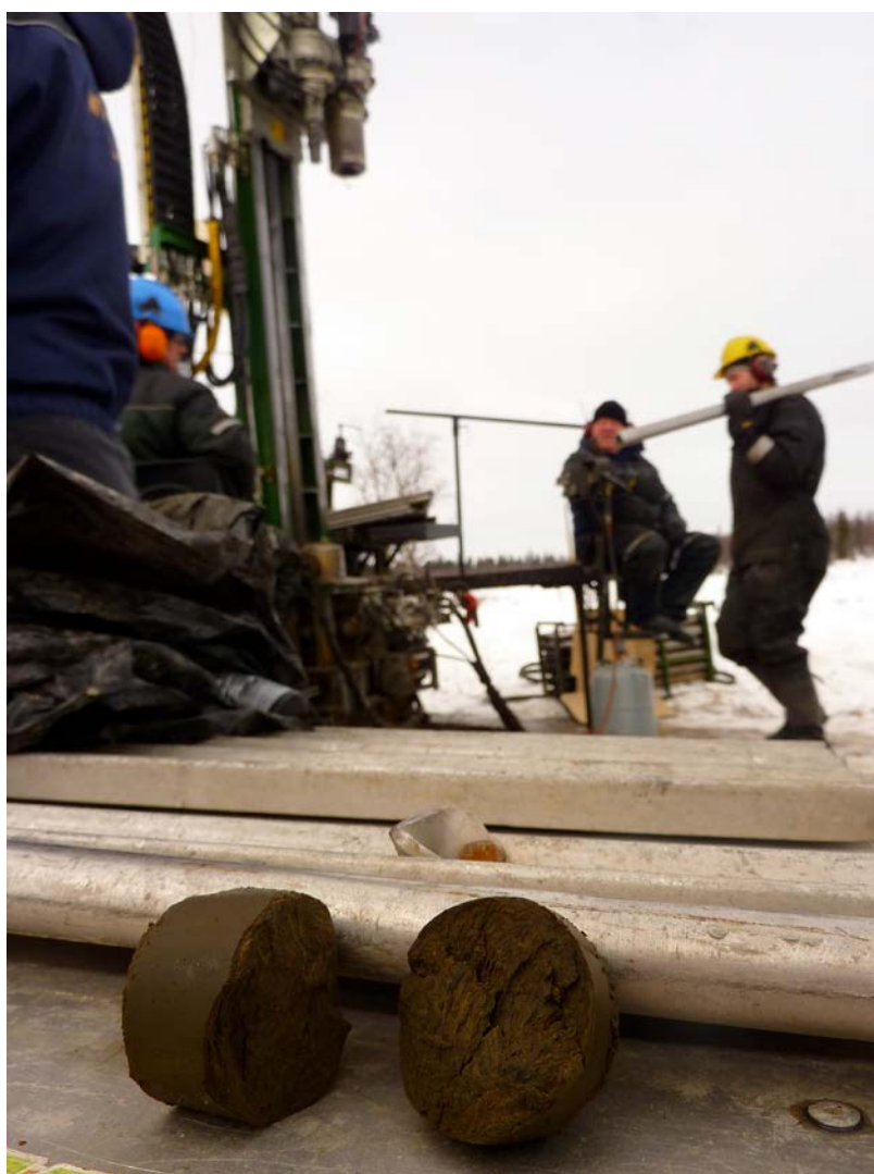
Figure 5-1. Drilling of the Sokli 2010/4 borehole by the Geological Survey of Finland. A core slice of the Eemian diatom gyttja sediment is shown in the foreground.
