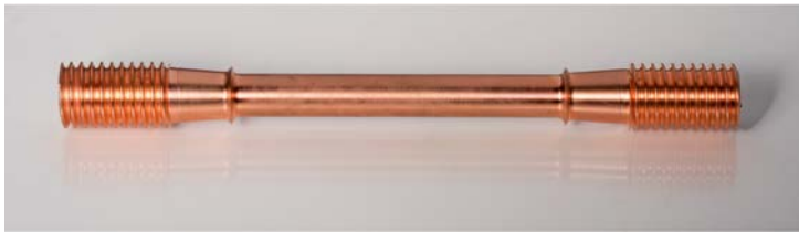
Figure 2-2. A manufactured creep test specimen.
