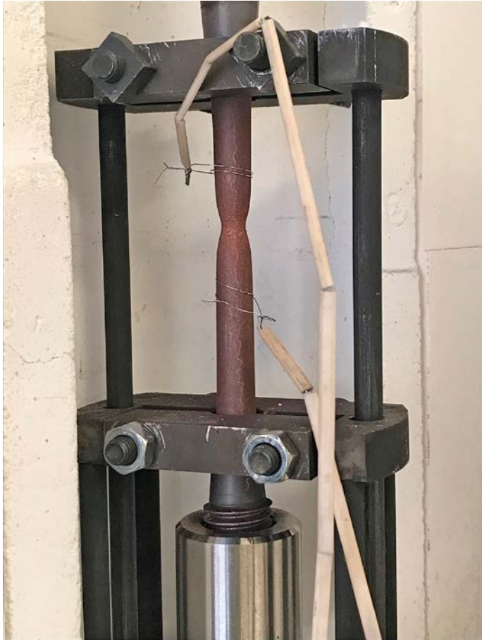
Figure 3-1. Approximate positioning of the thermocouples on the specimen. The thermocouples are tied to the specimen using a stainless steel wire.
