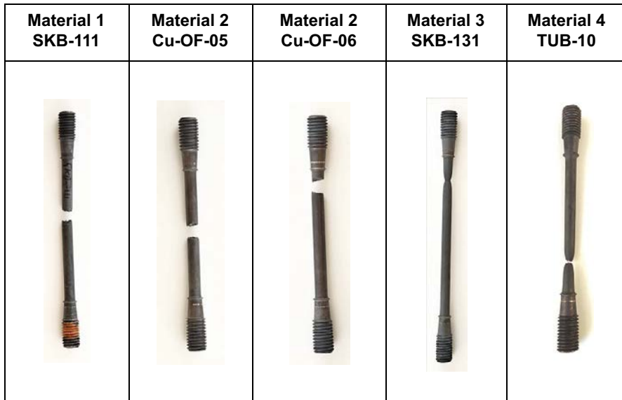
Figure 4-13. Specimens after SSRT testing at 215 °C.
