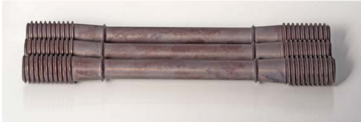
Figure 2-4. Creep test specimens after annealing.
