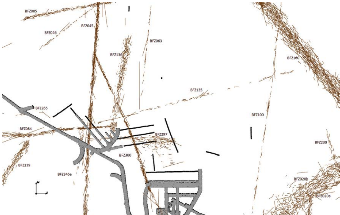
Figure 2-5. A slice at z = -420 m through the fault associated fractures (brown) around the base of the ONKALO shown on a scale of 800 m E-W. No sealed parts of the fractures are removed at this stage. This figure is reproduced from Hartley et al. (2018).
