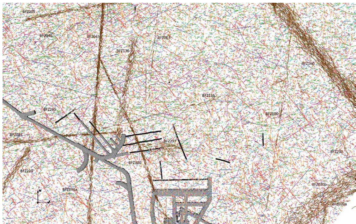
Figure 2-6. A slice at z = -420 m through the combined DFN model for fault associated fractures (brown) and the background fractures in the rock mass (see Figure 2-1). The slice is shown local to the base of the ONKALO on a scale of 800 m E-W. This figure is reproduced from Hartley et al. (2018).
