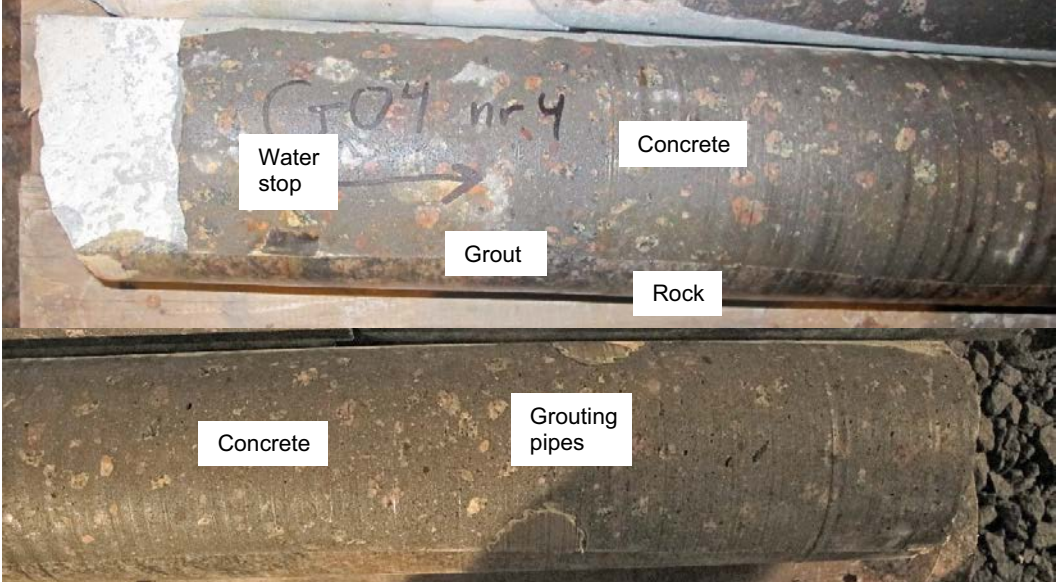
Figure 2-8. Examples of drill cores (G04) from the interface between rock and concrete immediately after drilling. The water stops (dark squares) and grouting pipes (light colored halve-circles) are clearly visible. Very little or almost no grout seems to have penetrated at the interface. These cores seemed to be attached to each other after drilling, i.e. a certain bond strength existed.
