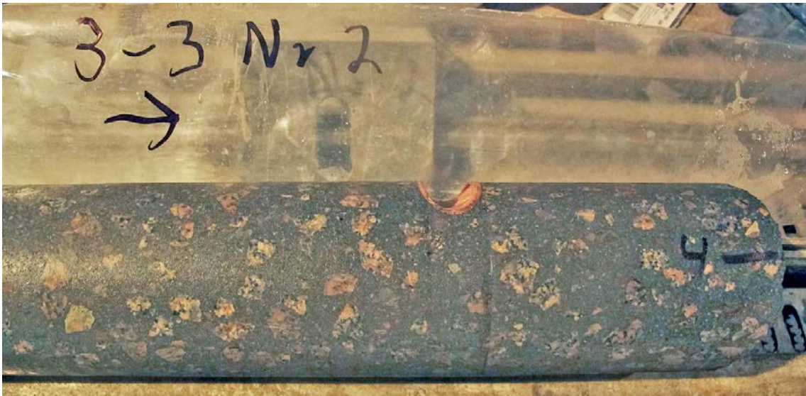
Figure 2-10. Core 3-3-1, part 2. The large aggregates seem very well distributed, the cooling pipe is well embedded in concrete.
