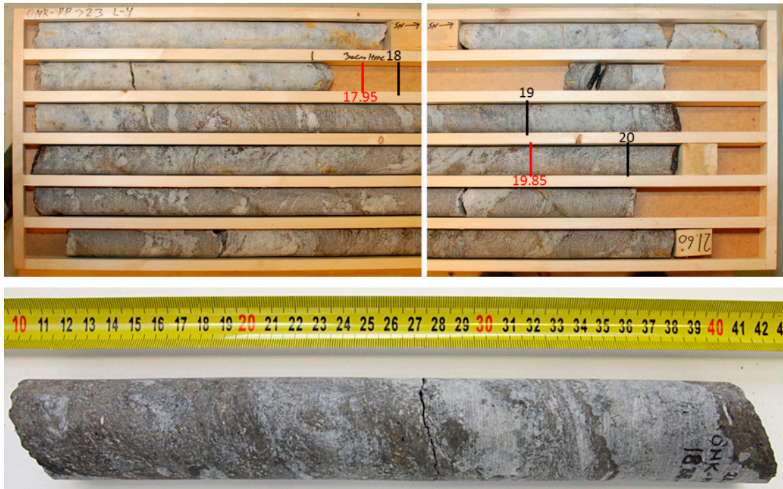
Figure 2-8. Drill core from the WPDE experimental section 17.95–19.85 m. Missing piece from 17.90–18.20 m was taken to the laboratory experiments before logging of the drill core, and is shown separately in the lower photo. All displayed fractures in the experimental section are judged to be mechanically induced (broken) in the core drilling, and there is no natural fracture. Photos from Helsinki University.
