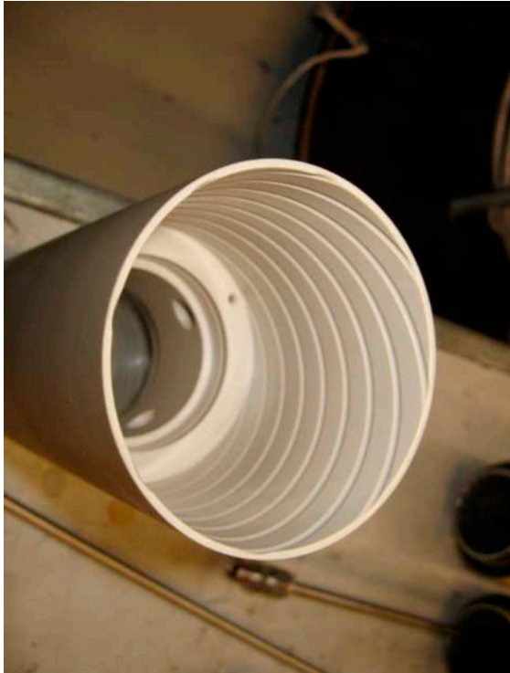
Figure 2-2. Grooves are applied on the equipment to facilitate the mixing of the injected tracer solution with the synthetic groundwater; rubber sealing is covering the grooves.
