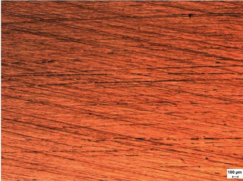
Figure 2-2. Coupon surface before exposure. The scale bar is 100 \mu\text{m} .
