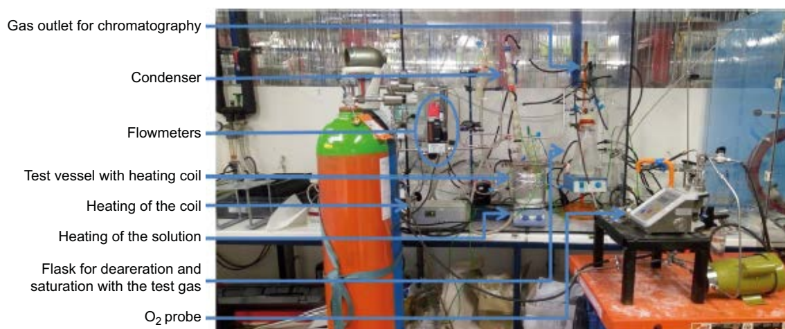
Figure 2-11. Overview of test set-up.
