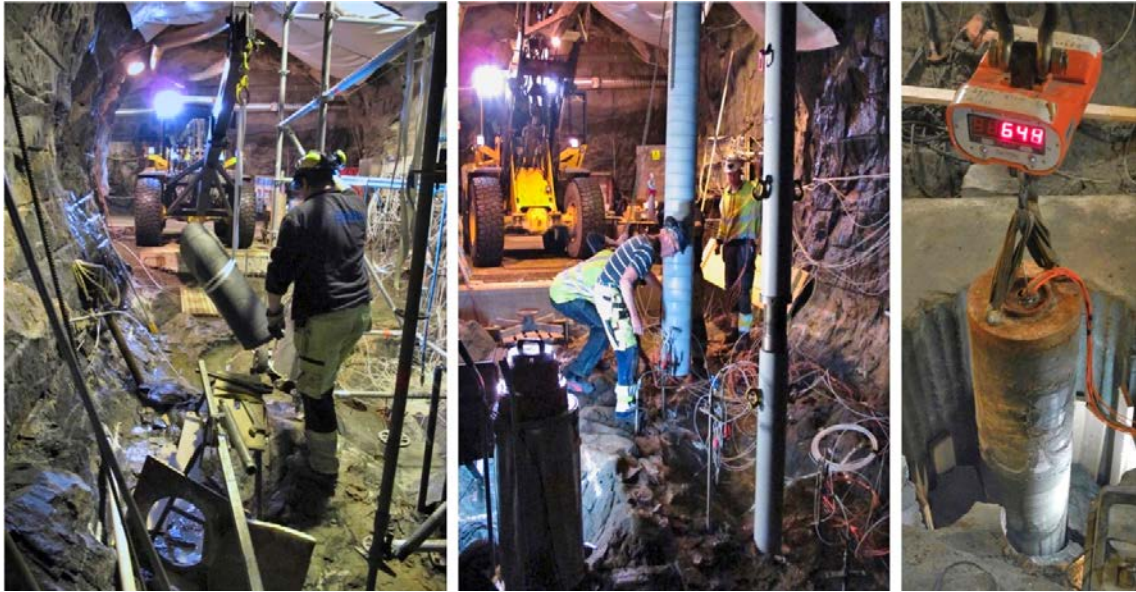
Figure 1-6. The BRIE site in the TASSO tunnel: drilling of the 300 mm boreholes (left), emplacement of the 3 m bentonite blocks (middle), extraction of bentonite blocks after 17 months (right) (Fransson et al. 2017).
