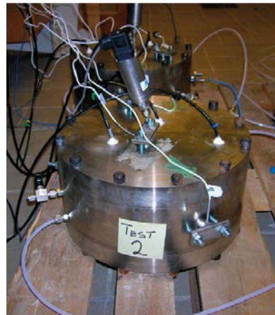
Figure 1-8. a) Schematic and b) photograph of the BRIE water-uptake test. Water is introduced via the outer cylindrical filter. The 100 mm bentonite block is identical in material to the stack of blocks employed in the BRIE in situ experiments (Vidstrand et al. 2017, Fransson et al. 2017).
