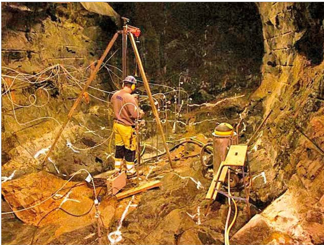
Figure 1-2. a) Boreholes in tunnel wall and location of BRIE test bed; b) probing holes; boreholes KO0017G01 and KO0018G01 had their diameters increased from 76 to 300 mm, becoming “surrogate deposition holes”; c) BRIE test bed in TASSO tunnel (Fransson et al. 2017).
