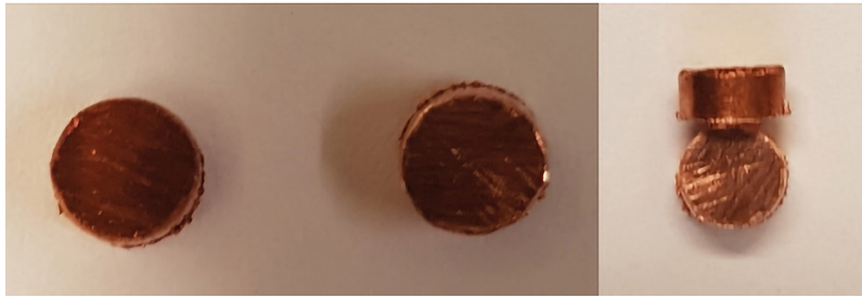
Figure 2-2. Discs cut from the top and bottom of each Cu rod.
