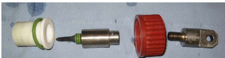
Figure 2-7. Parts of the SSRT-cell, dismantled. Lower, stationary side of the test rod after testing.
