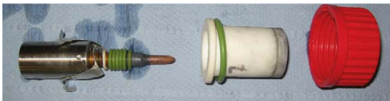
Figure 2-6. Parts of the SSRT-cell, dismantled. Upper, moving side of the test rod after testing.
