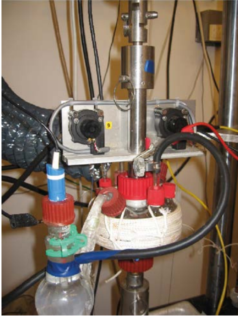
Figure 2-4. Photograph of the SSRT-cell with a mounted test rod.
