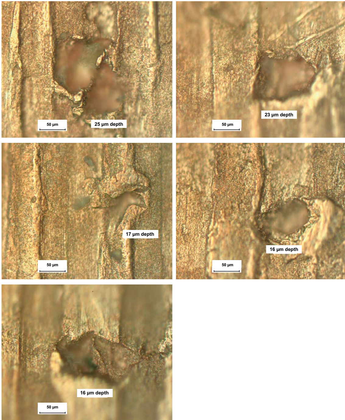
Figure 3-4. Microscope images of the five deepest defects found on Specimen 18.
