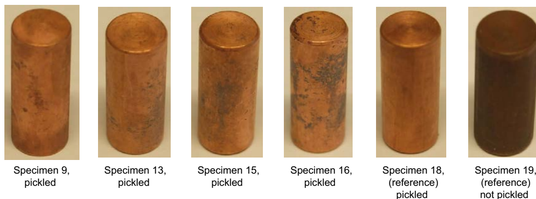
Figure 3-2. Corroded copper specimens after pickling. Reference specimens pickled and not pickled.
