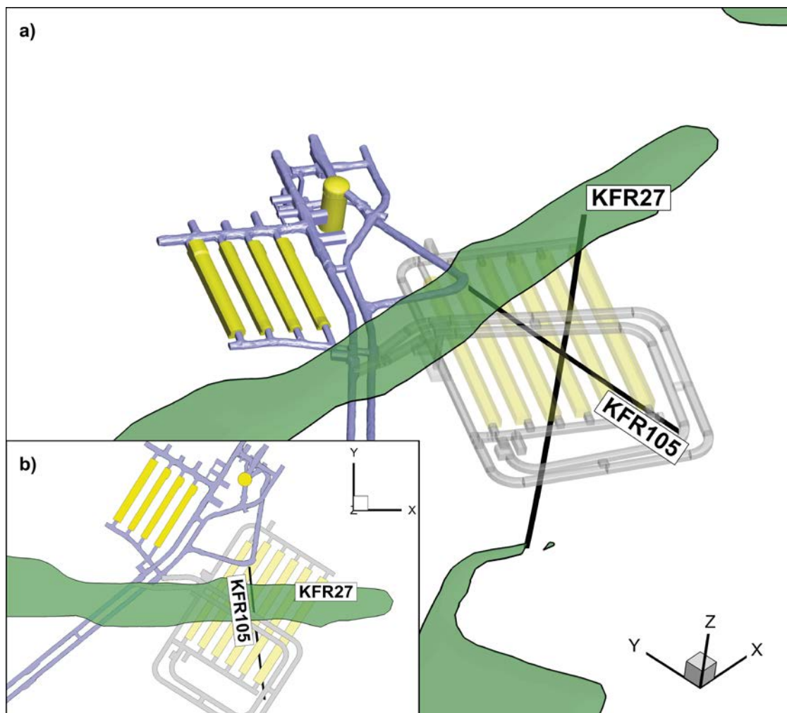
Figure 1-1. The investigated boreholes, KFR27 and KFR105, in Forsmark in relation to existing SFR (yellow) and planned extension (grey) seen from an angle (a) and straight from above (b). Borehole KFR105 is situated in the SFR-tunnel at about 106 m depth and KFR27 is drilled from the surface.
