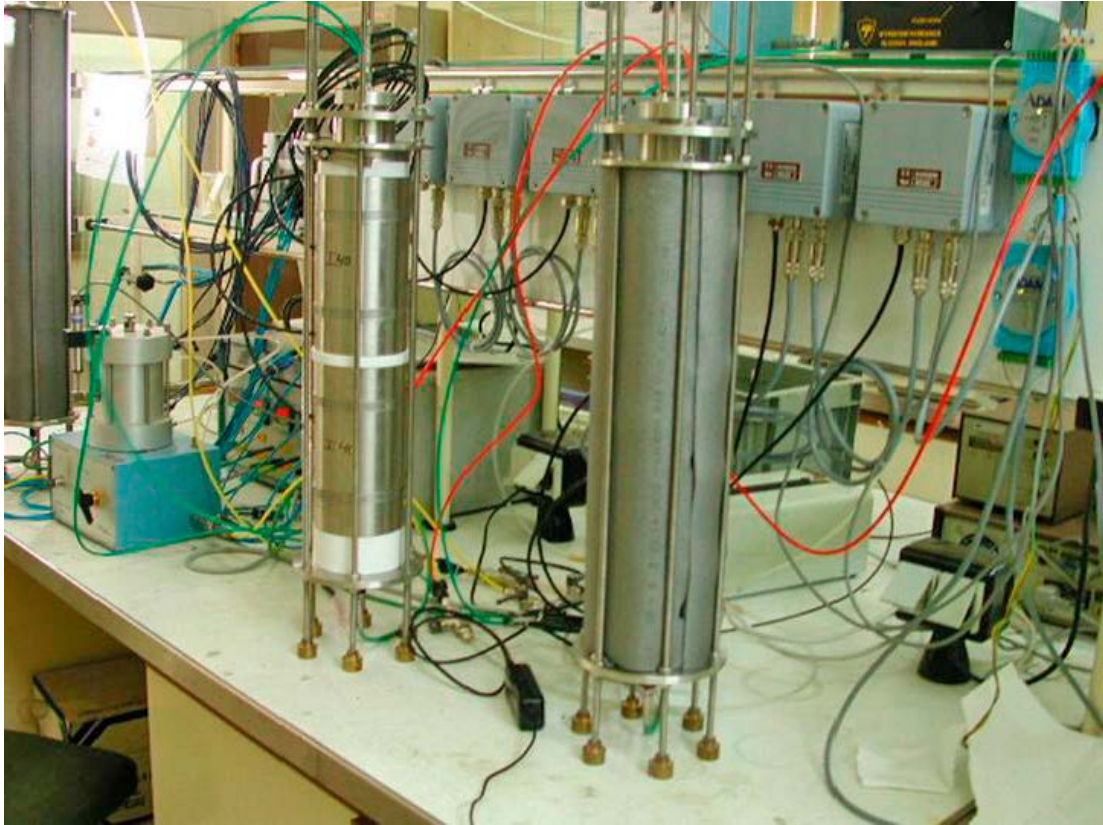
Figure B-1. Large infiltration cells: isothermal test (left) and thermal gradient test (right).
