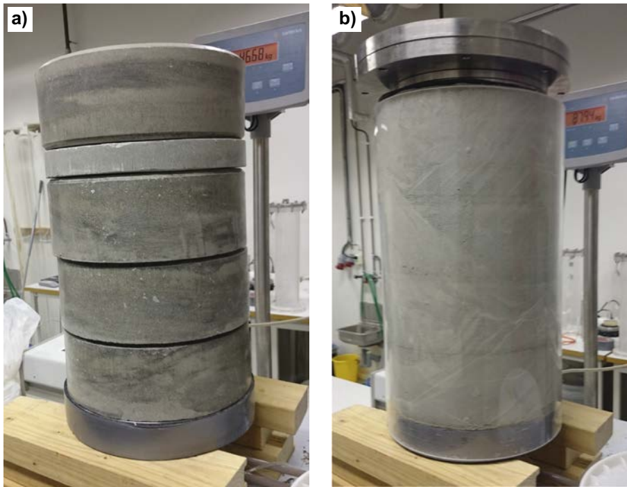
Figure 3-2. The configuration of the most recent test, Test 9: a) Four bentonite rings and a massive block stacked on top of each other, b) The full set-up before starting the experiment. (Birgersson and Goudarzi 2017).
