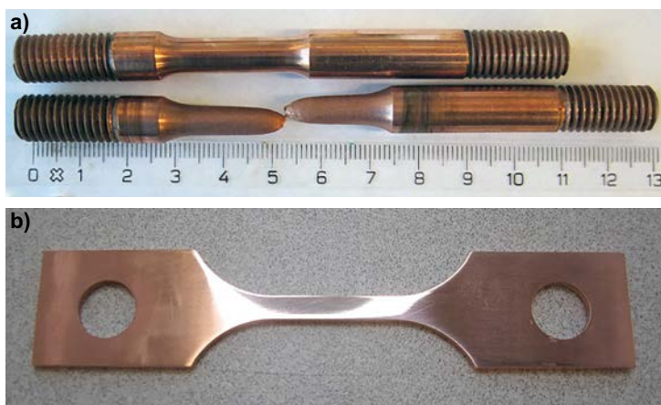
Figure 6-1. Examples of tensile specimens used for slow strain rate testing (SSRT), a) round specimens, before and after drawn to rupture, b) a flat rectangular specimen (Taxén et al. 2018).
