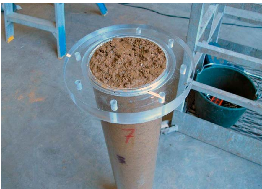
Figure 7-7. Asha pellets installed in a simulated water filled borehole. The photo is taken during test termination.
