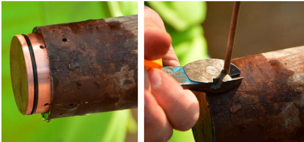
Figure 11-3. Left: Installation of the end plug made of copper. Right: Mounting of the shear rods.
