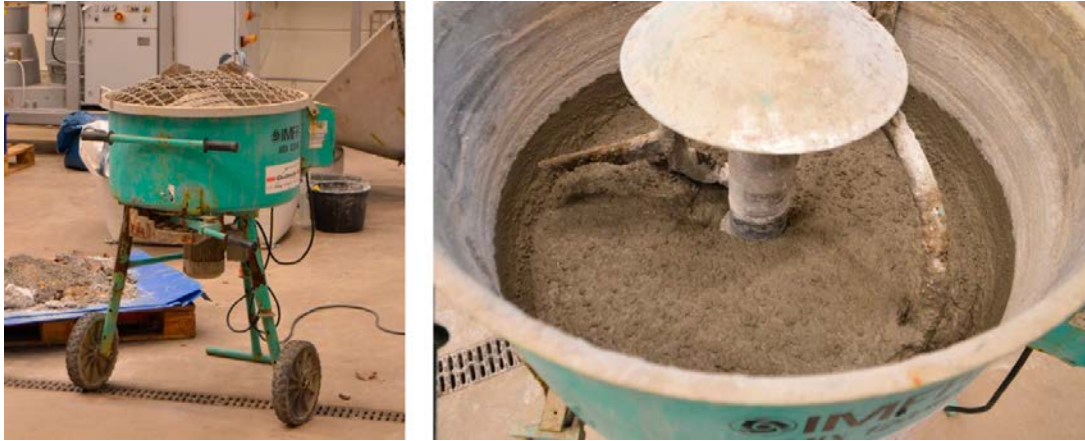
Figure 11-1. The forced concrete mixer used for mixing the concrete.
