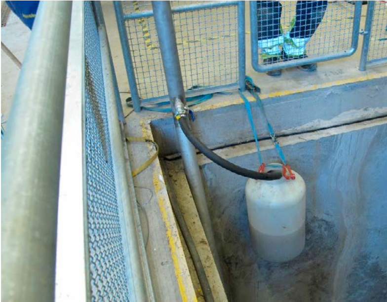
Figure 8-2. Photo showing the arrangement for collecting outflowing water from the simulated borehole.
