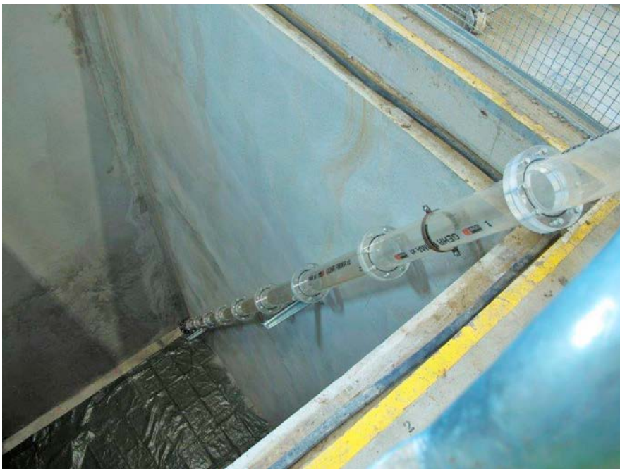
Figure 7-3. Photo showing the test setup for the tests performed simulating inclined boreholes.
