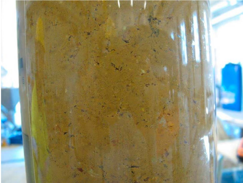
Figure 7-8. Photo showing Asha pellet installed in a simulated water filled borehole.
