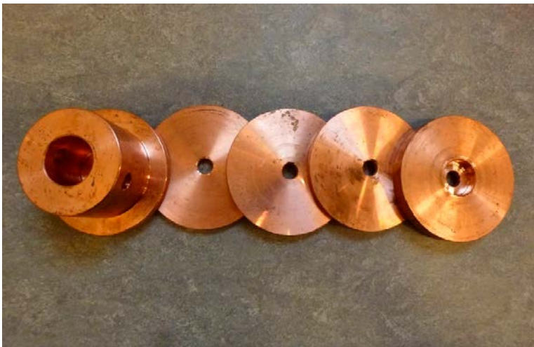
Figure 12-4. Photo showing the copper parts included in one bentonite package.
