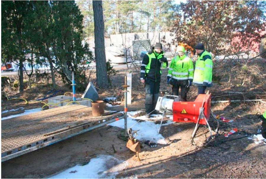
Figure 9-2. Photo showing the measuring cable equipped with a camera in the end.
