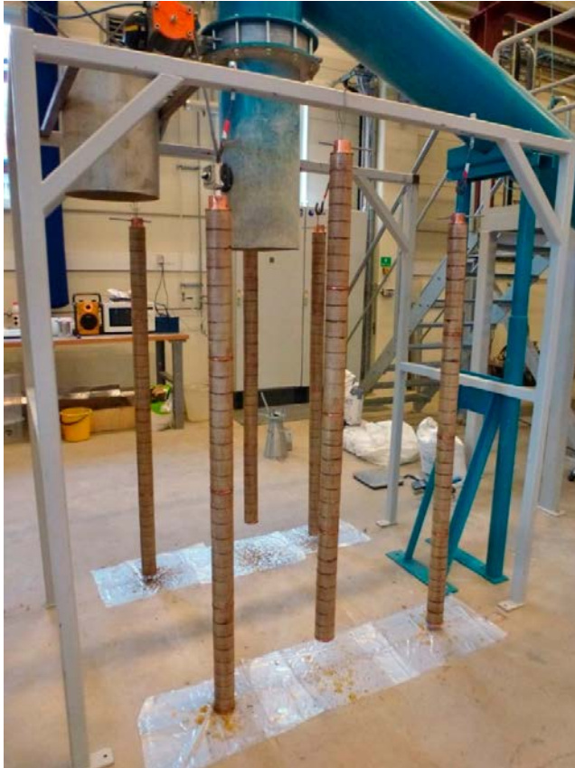
Figure 12-5. After assembling of the bentonite packages, they were hanged up and painted with shellac.
