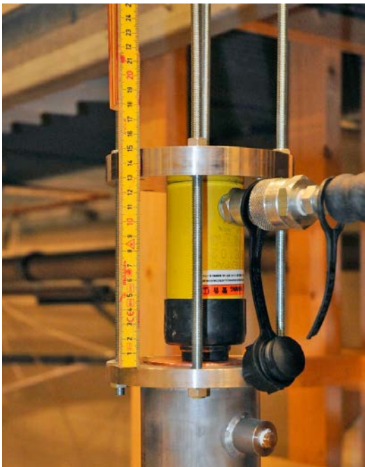
Figure 6-6. A hydraulic piston was used to compress the copper expander.
