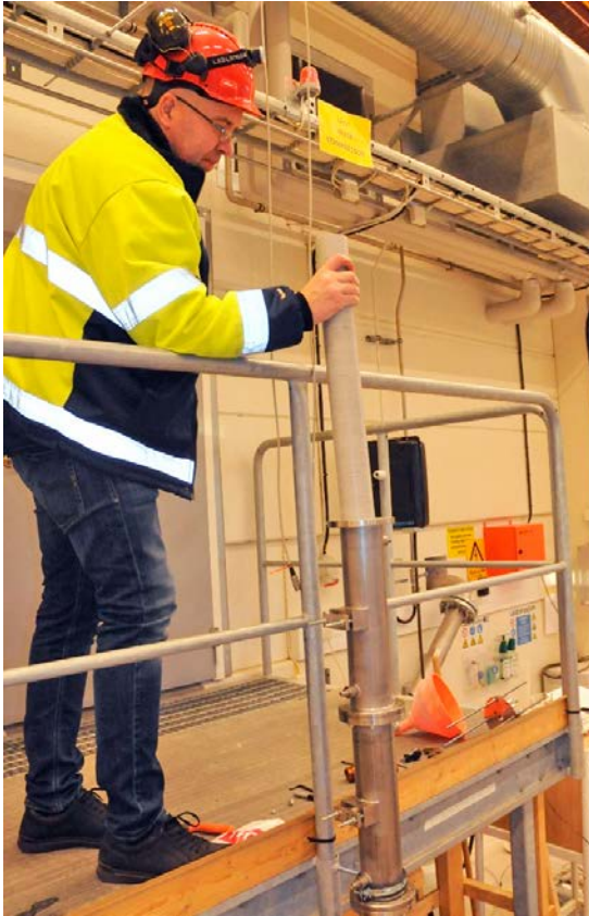
Figure 6-8. Left: Installation of one of the bentonite packages. Right: Three sensors (left side of the tube) are registering the radial swelling pressure from the bentonite section.
