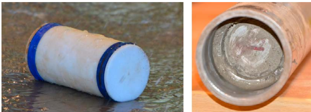
Figure 11-4. Left: The piston made of nylon with its seals. Right: The welded ring inside the special drill tube that is preventing the nylon piston from falling into the borehole.
