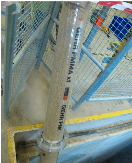
Figure 7-5. Close-up showing pellet installation in a simulated dry borehole.
