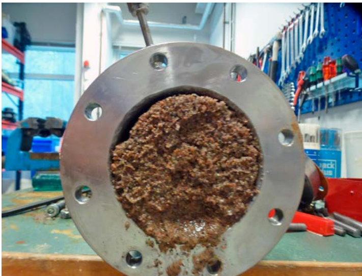
Figure 6-19. Photo showing the sand filling from the lower section during excavation.
