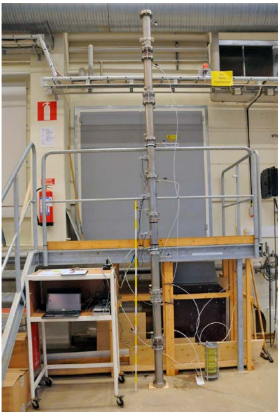
Figure 6-9. Overview of the test setup after having finished the installation. The vessel on the floor to the right contains the pressurized water.
