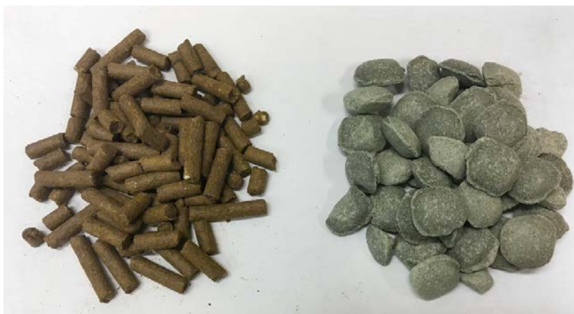
Figure 7-1. Photo of the two pellet types used in the tests. Left: Asha pellets Right: MX-80 pellets.
