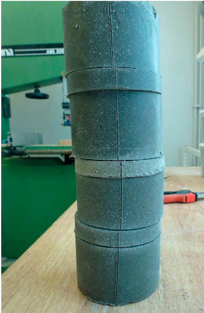
Figure 5-7. Photo of the bentonite core. The different sampling sections have been cut out and then piled on each other.
