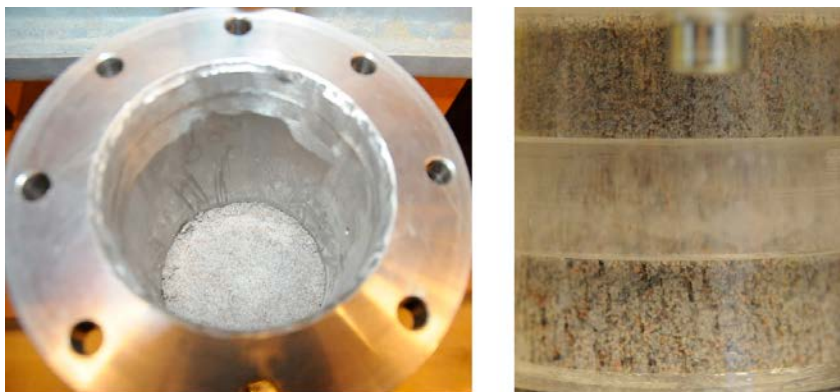
Figure 6-7. Left: Top of the quartz based concrete section after about one day curing. Right: Close-up of the quartz-based concrete through one of the Plexiglas sections. The band that crosses at the mid-height of the photo is an extra reinforcement made of Plexiglas.
