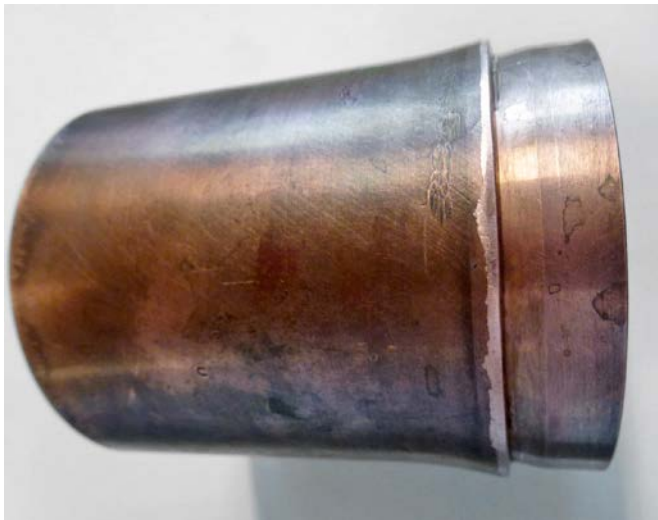
Figure 6-20. Photo showing a copper expander after extrusion from the test cell.
