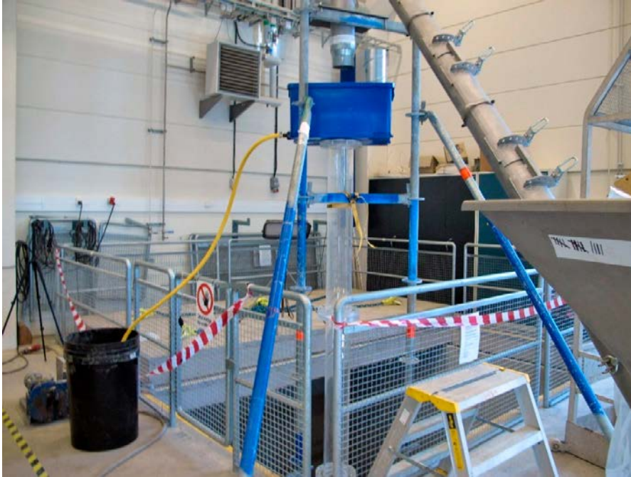
Figure 7-6. Photo showing the test setup for the tests including a simulated water filled borehole.
