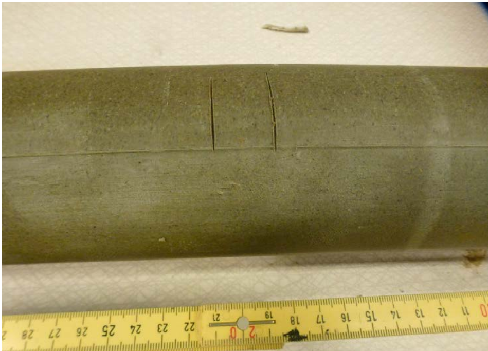
Figure 6-15. Photo showing a part of the bentonite sealing after extrusion from the test cell.
