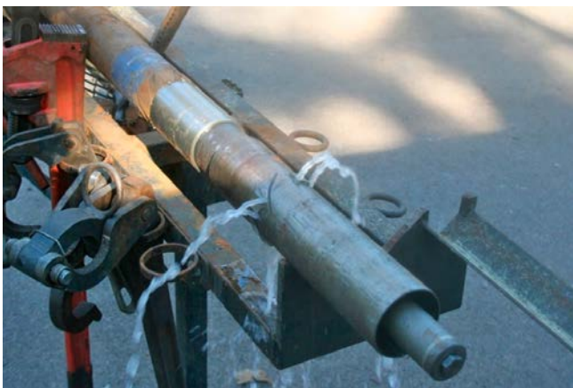
Figure 12-9. Photo showing the reaming tool used to increase the borehole diameter at two levels.
