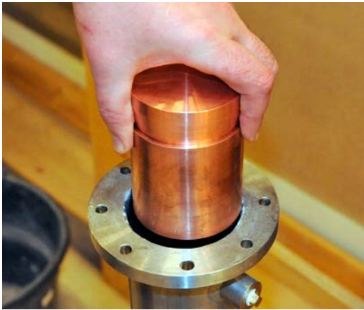
Figure 6-5. Installation of a copper expander in the simulated borehole.
