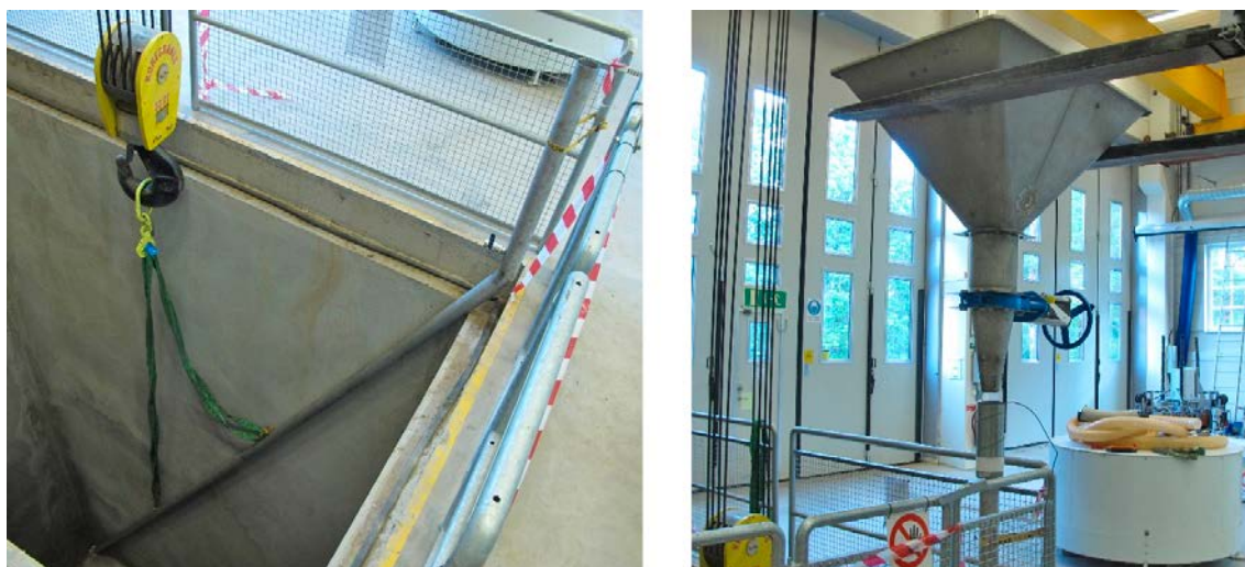
Figure 8-1. Photo showing sand installation in a simulated borehole.
