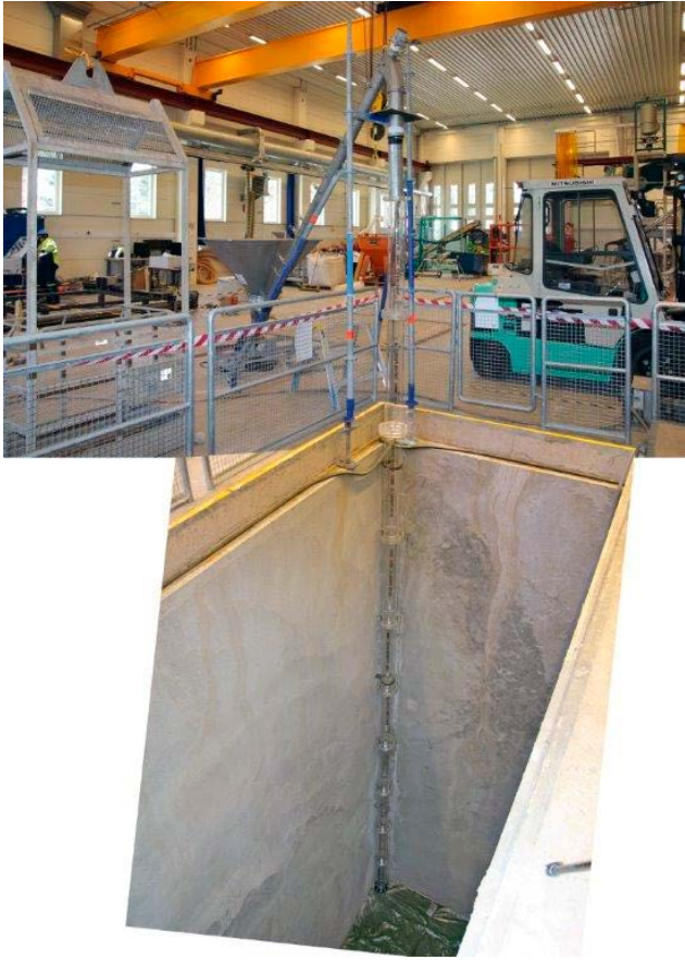
Figure 7-2. The simulated borehole (length = 10 m) is placed in an eight-meter-deep shaft in the laboratory (photo collage).
