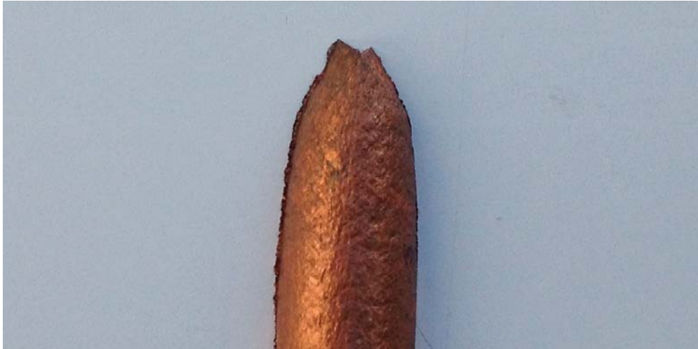
Figure 4-2. One end of a failed cylindrical Cu OFP creep specimen; note the extreme level of necking. The specimen is split alongside, thus the burrs at the edges.
