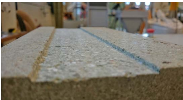
Figure 4-4. Milled track in bentonite.
