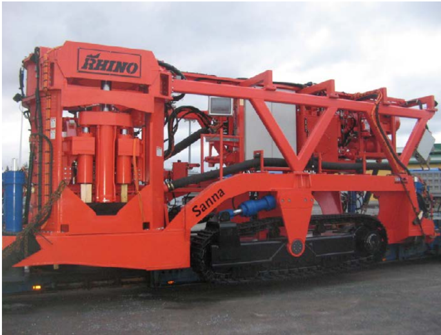
Figure 3-12. Prototype deposition hole drilling machine used by Posiva.
