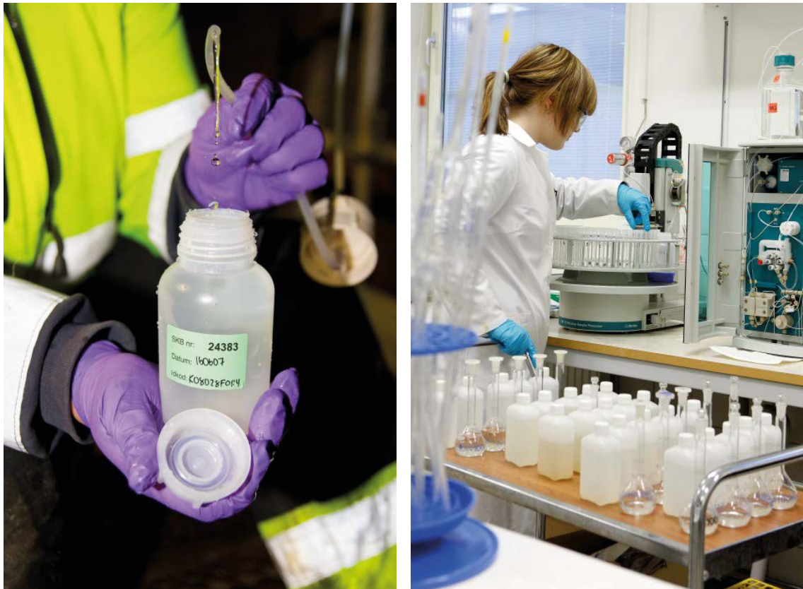
Figure 2-5. Ongoing sampling of ground water from packed-off sections (left figure) and analysis of anions at the Äspö chemical laboratory from collected water (right figure).
