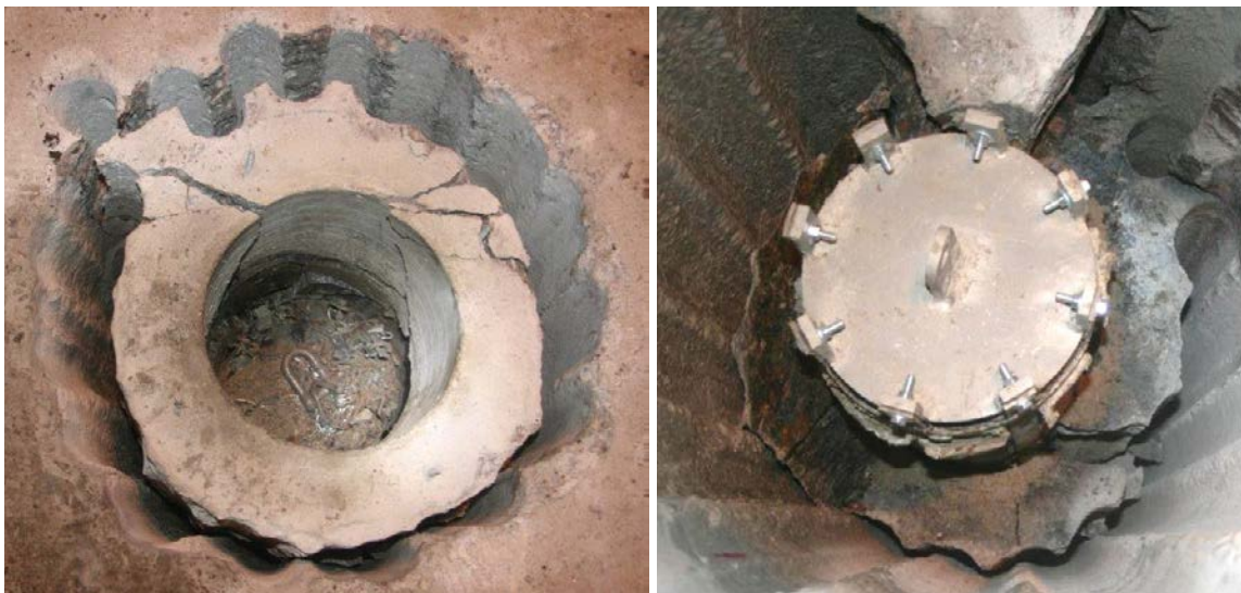
Figure 3-24. Over coring of experiment #20 and removal of the fractured rock from the deposition hole.
