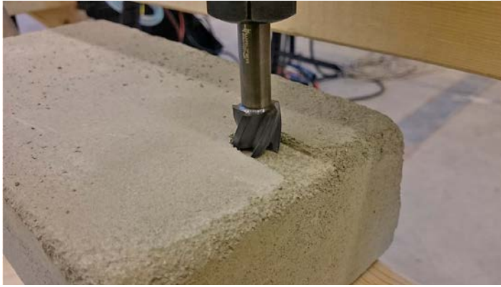
Figure 4-3. Motor spindle milling in bentonite.
