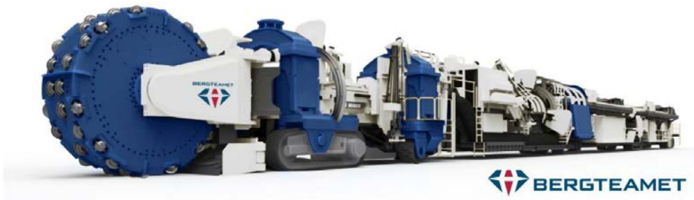
Figure 3-3. TBS also referred to as Mobile Miner planned to be tested at Äspö during 2018.
