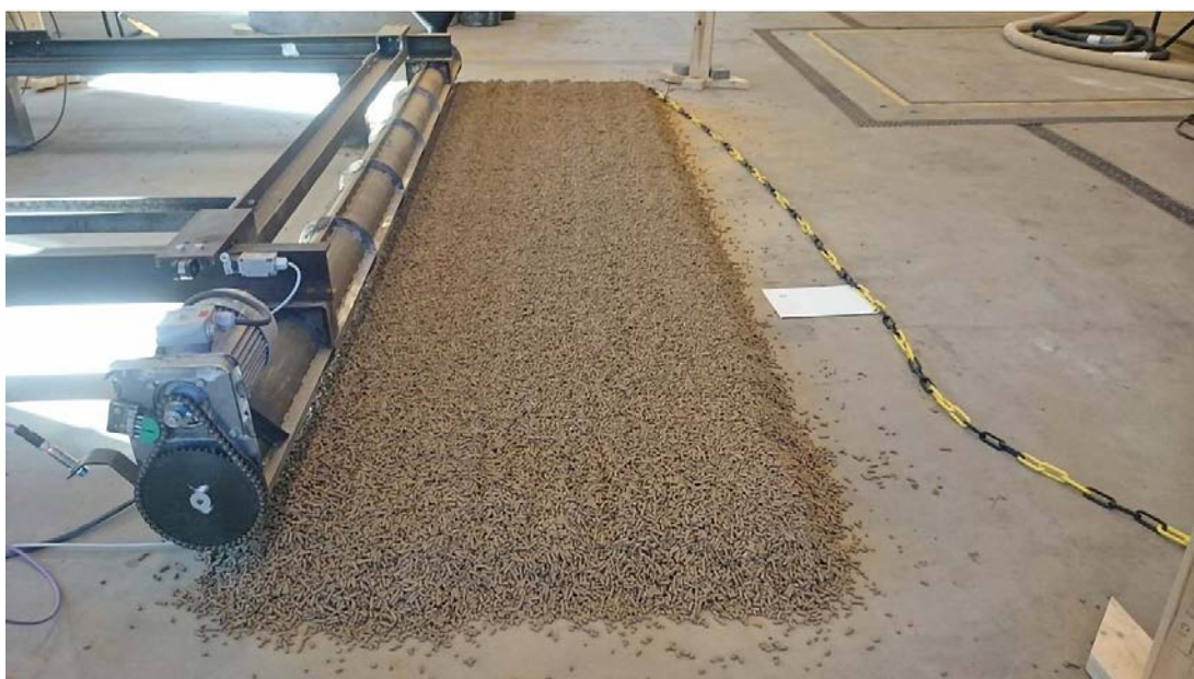
Figure 4-6. Pellet layer being produced during test.
