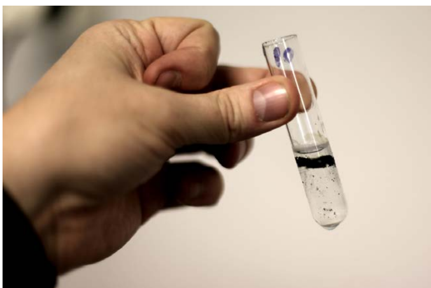
Figure 5-2. Sulphide (in the form of CuS) formed by microbiological activity of sulphate reducing bacteria from gypsum in the presence of liquid water. Gypsum is a common mineral in bentonite, and this sulphate to sulphide transformation is the subject of the study.
