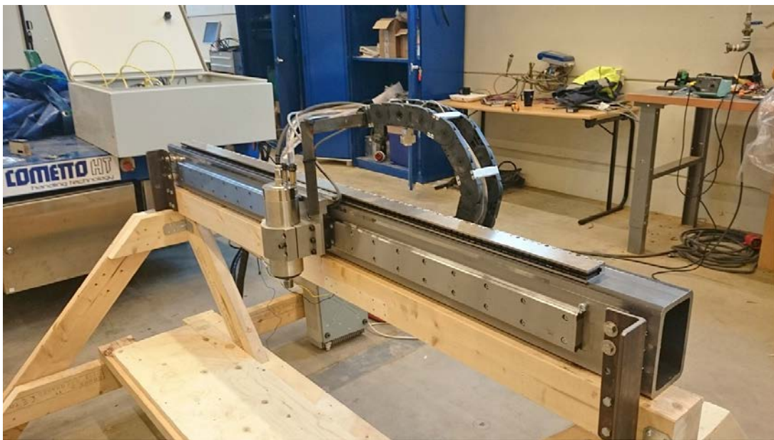
Figure 4-2. Test rig for the linear motor and the motor spindle.
