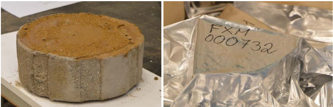
Figure 3-26. One of the bentonite blocks, prior to segmentation (left image) and after segmentation and packaging (right image).
