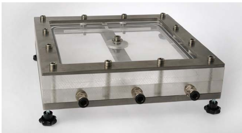
Figure 5-1. Experimental cell for measuring of chemical erosion of different bentonites.
