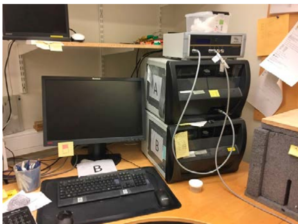
Figure 4-1. TPS-apparatus TPS 2500s with sensor switch.
