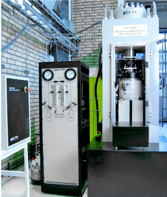
Figure 4-4. Rock testing system. From left: Digital controller unit, pressure cabinet (used for triaxial tests) and load frame. The PC with the test software (not shown in the picture) is placed on the left hand side of the controller unit.
