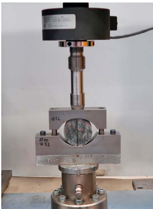
Figure 4-3. Test-set up for the indirect tensile strength test. The load cell is visible in the top and the curved bearing blocks are seen below that.
