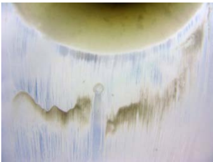
Figure 2-10. Close-up photographic image of test with a 50/50 mix of CaMt and NaMt at 90° rotation from a horizontal fracture position to vertical.
