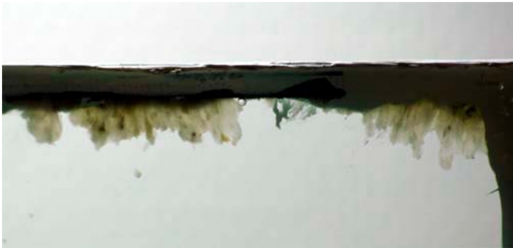
Figure 2-5. Upside down turned sediment in 1 mm aperture fracture 24 hours after turning the slot upside down. Floc fingers are slowly pulled downward by gravity. Small flocs are released and very slowly move downward. The whole picture is about 4 cm high.
