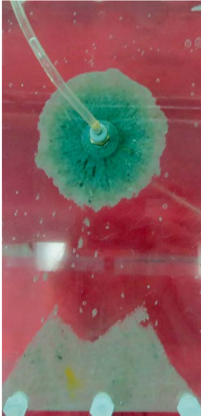
Figure 2-12. Image of extrusion and mass loss of Wyoming bentonite in a 45° sloped fracture after 720 h. The test was conducted in a 1 mm aperture fracture filled with stagnant water with 0.68 and 0.14 mM, Na + and Ca 2+ respectively. The sample was initially emplaced at a dry density of ~1.6 g/cm 3 (Schatz and Akhanoba 2017).
