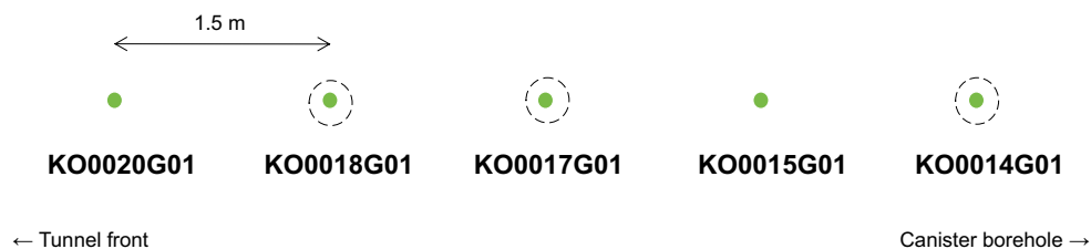
Figure 2-5. Illustration of probe borehole spacing and naming. The dotted lines indicate proposed overcoring of the selected probe boreholes. This figure is reproduced from the task description (Vidstrand et al. 2017).
