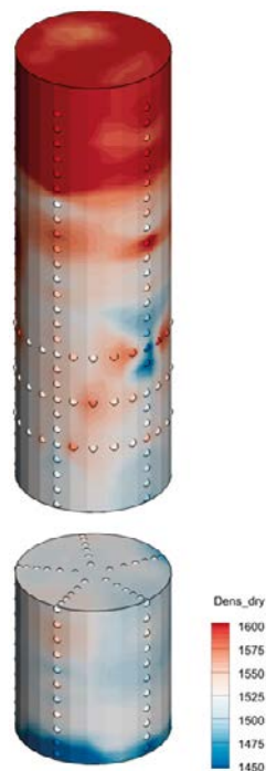
Figure 6-21. The dry density of bentonite in hole 17 after dismantling. Figure by Mattias Åkesson.
