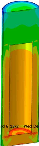
Figure 7-4. Void ratio (upper) and dry density ( \text{kg/m}^3 ) in the buffer.
