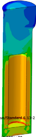
Figure 9-5. Average effective stress (upper) and vertical total stress (kPa) in the buffer.
