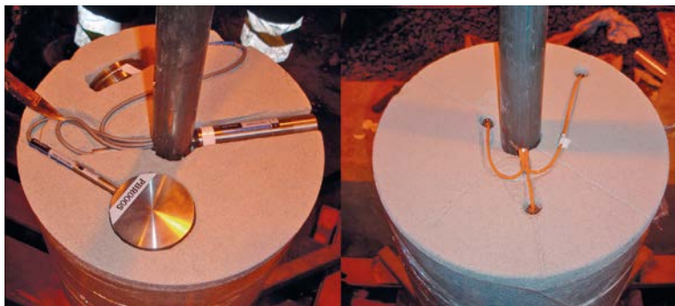
Figure 5-1. Position of the sensors between two bentonite blocks (Fransson et al. 2017).
