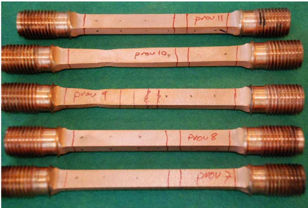
Figure 8-1. The creep test specimens after testing. The pieces marked by the parallel red lines are the material extracted for metallography.
