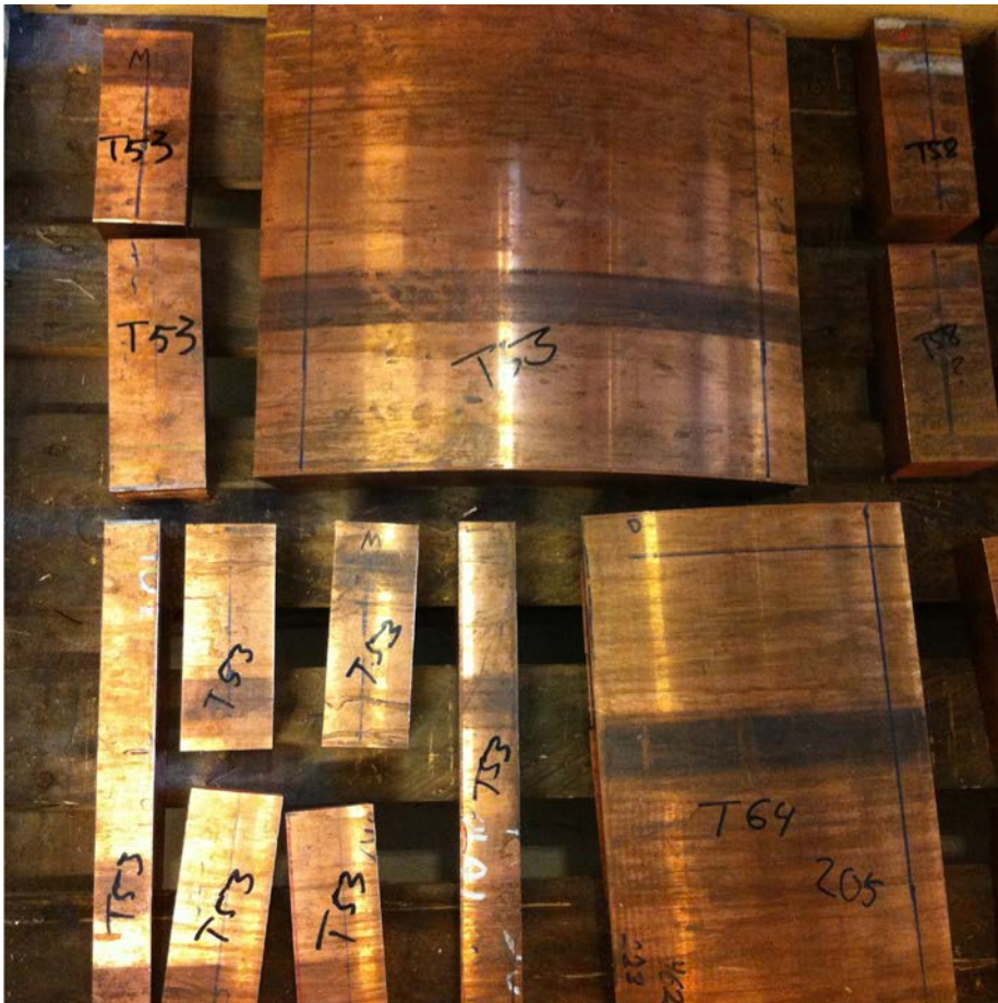
Figure 6-1. The material used for the creep testing as delivered. The studies pieces are from the T58 material visible in the upper right corner. The image was taken during the work described in Mannesson and Andersson-Östling (2013).
