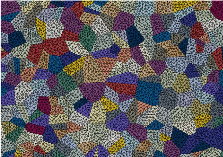
Figure 5-3. A small section of the finite element mesh of the polycrystal using a single grain size distribution.
