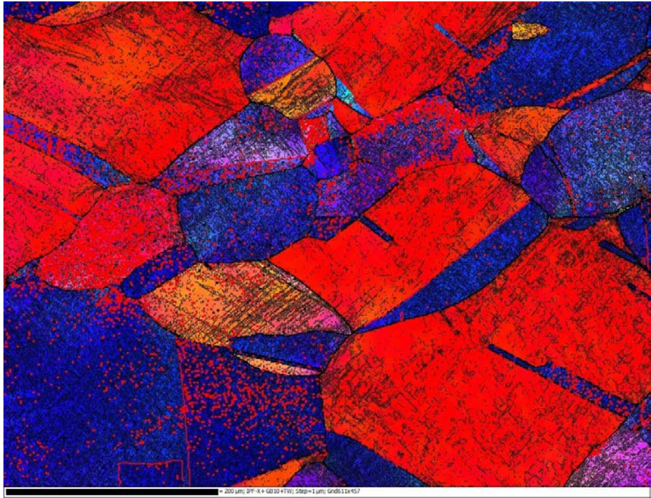
Figure 8-10. High angle boundaries (thick black) and low angle boundaries (thin black) in specimen 11. Low angle boundaries are associated with the grain substructure and the density is a measure of the strain in the grain.
