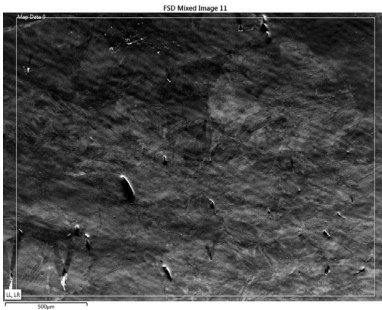
Figure 8-11. SEM image from specimen 15-11. This specimen is made from Cu-OF from a previous creep test study.
