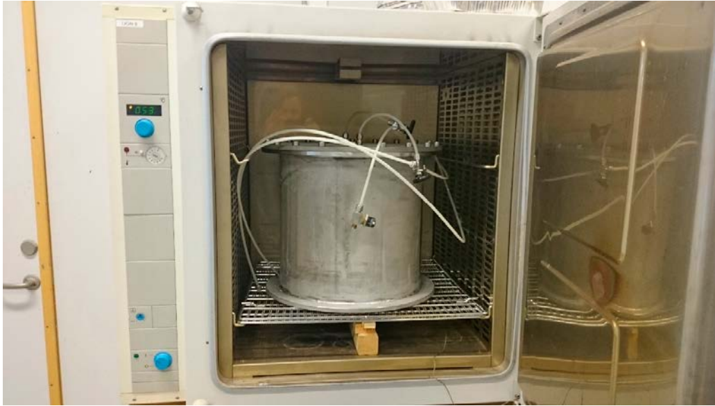
Figure 2-5. The isothermal test placed in the oven.
