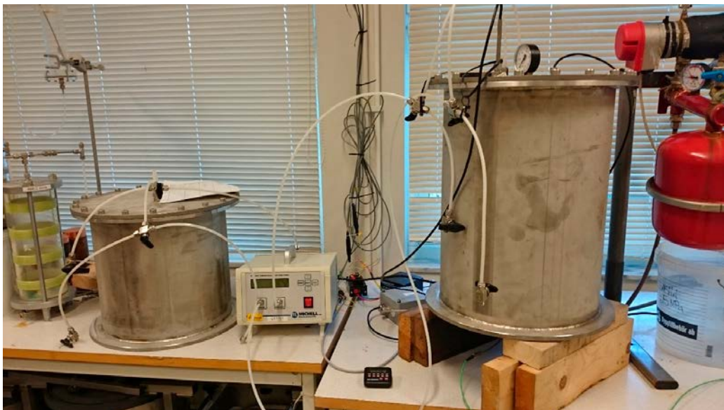
Figure 2-6. The isothermal (left) and thermal gradient (right) tests under operation in the lab. In the middle of the picture is seen the oxygen analyser (at the time of the photograph, connected to the thermal gradient test). To the far right is also seen the water heating system.
