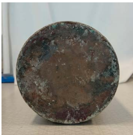
Figure 3-9. Top of the heater in the thermal gradient test after termination. A black corrosion product ( \text{CuO} ) is seen in the upper part, a red corrosion product ( \text{Cu}_2\text{O} ) is visible in the lower part.
