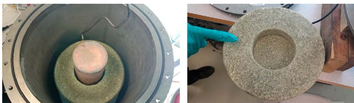
Figure 2-4. Left: Assembly of the blocks and rings. In this picture is also seen the titanium tubing for the RH-sensor located close to the heater. Right: Bottom side of the top block in the thermal gradient test. This block has a milled hole for fitting the top of the heater.
