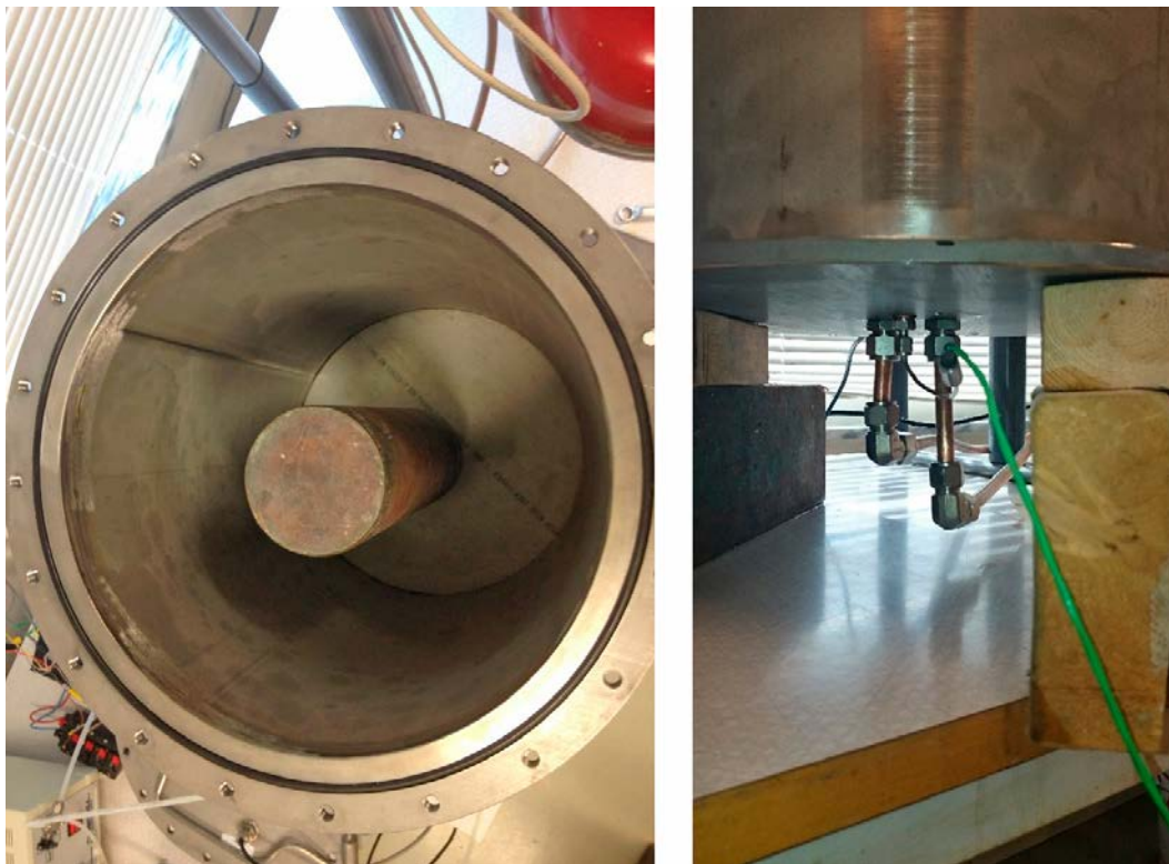
Figure 2-3. The copper heater assembled in the thermal gradient test. The photograph to the right shows the connection at the bottom of the “barrel” for flowing heated water. The water heater is seen in Figure 2-6. The green cable seen in the right picture is for the thermocouple controlling the heat regulation.
