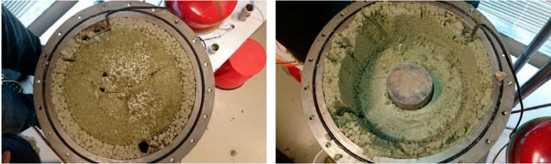
Figure 3-5. Left: Temperature gradient test after removing the lid at termination. In the top is seen the cable and tubing for one of the RH-sensors, in the middle is seen the two holes where tubes were inserted for gas sampling in the slot region between heater and bentonite. At the bottom is seen a hole where the other RH sensor were located (it was pulled out during opening). Right: After removing the top block. The top of the copper heater is exposed, the homogenization of the top of the pellets slot is clearly seen.
