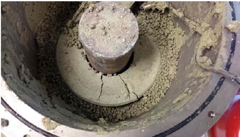
Figure 3-6. Sampling at the level of the mid-ring. The pellets slot was considerably dryer and less homogenized at this level in comparison with the top part. In the top right of the photograph is seen the RH-sensor which was located in this particular bentonite block during operation.
