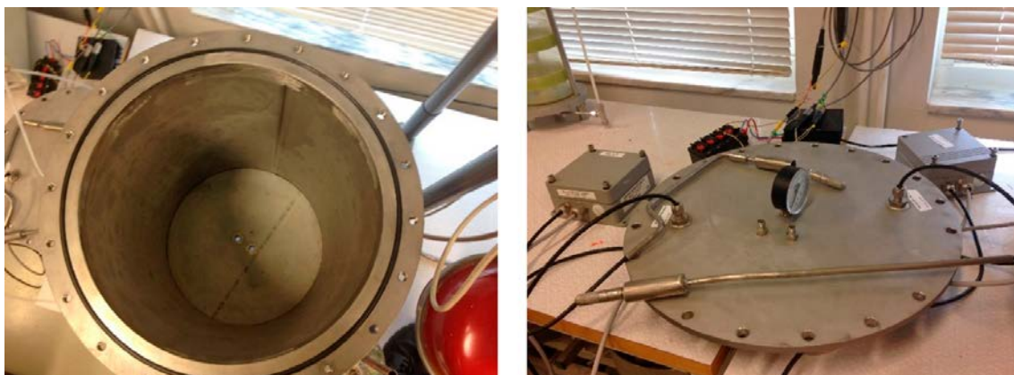
Figure 2-2. The container of the thermal gradient test. Left: the “barrel” seen from the top. The holes for inlet and outlet of heating water are visible. Right: The lid with the RH sensors and the total pressure gauge attached.
