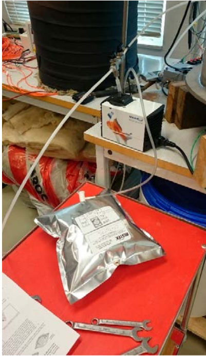
Figure 3-4. Gas sampling of the temperature gradient test. A vacuum pump was connected to one of the outlets of the tests and to the sample bag.
