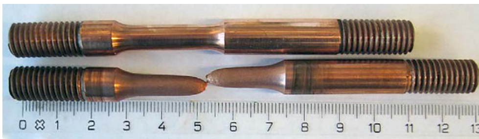
Figure 2-7. A photo of a new test rod and a test rod drawn to fracture in artificial seawater, for a reference curve.
