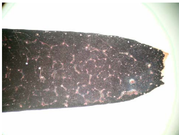
Figure 1-11. Apparent granular network on a polished, unetched surface of sample exposed in 0.414 M NaCl+1.56 mM Na 2 S+0.78 mM Na 2 S 2 O 3 at room temperature. The gauge diameter was 3 mm. (Bhaskaran et al. 2013.)
