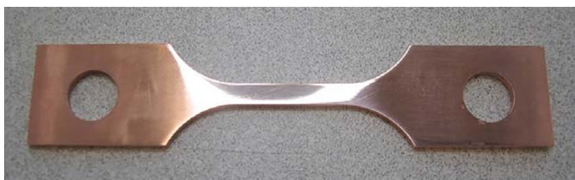
Figure 2-8. A photo of a rectangular test rod rectangular test rod before testing.
