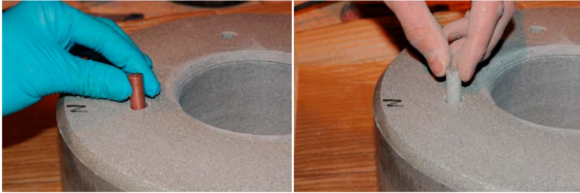
Figure 9-2. Left: installation of copper specimen in a pre-drilled hole Right: The hole is sealed with a cylinder manufactured of the same bentonite as the block.
