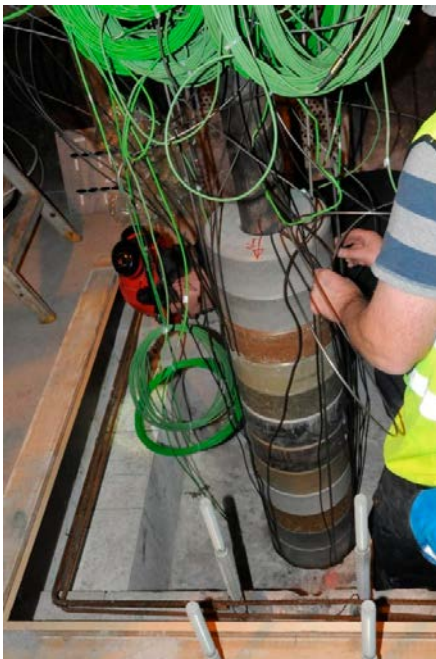
Figure 10-4. The test packages were lowered down into the holes very carefully.
