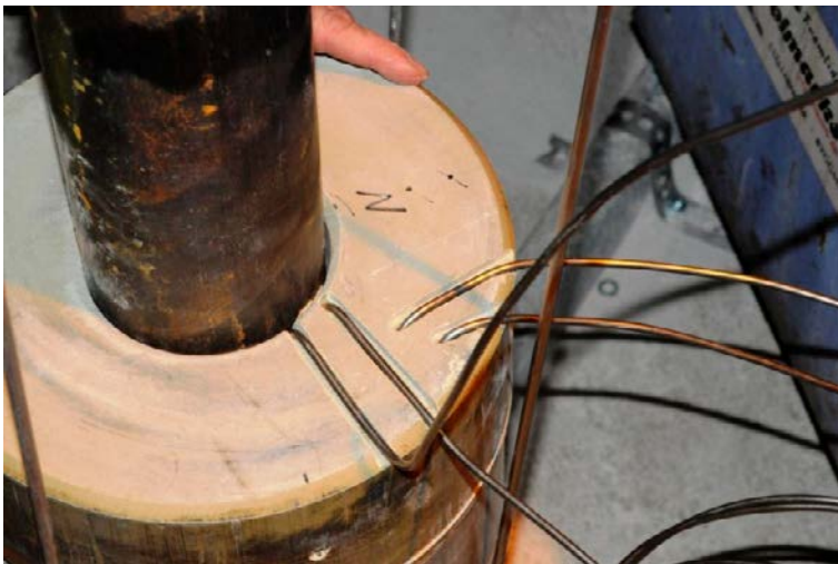
Figure 8-1. Photo showing the installation principle of thermocouples.
