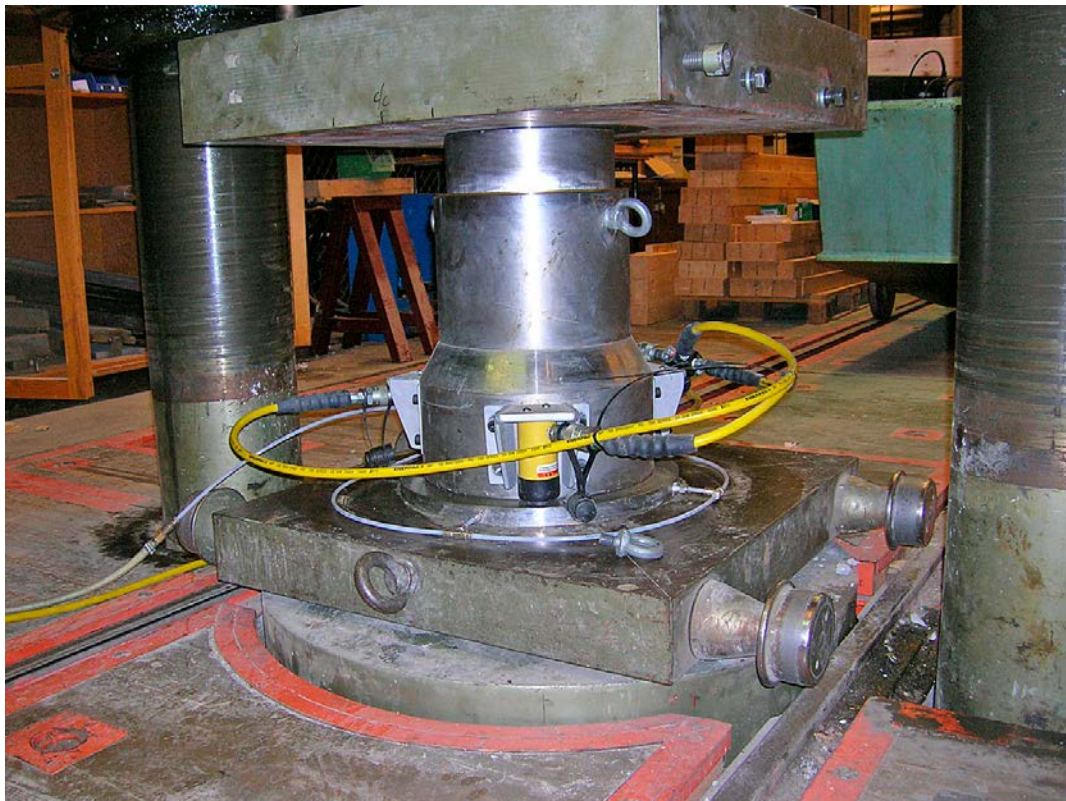
Figur 5-1. Photo showing the mould positioned in the press.
