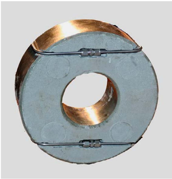
Figure 7-1. Photo showing the titanium tubes used for the artificial wetting and how they are connected to each other beneath the lowest block.
