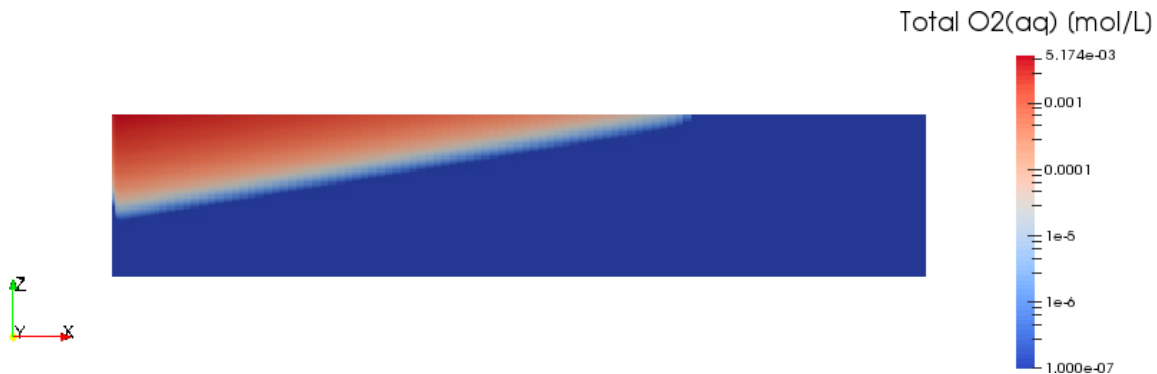
Figure 7-34. Oxygen concentration computed using iDP after 200 days of simulation time. The domain is magnified by a factor of 400 in the direction perpendicular to the fracture.
