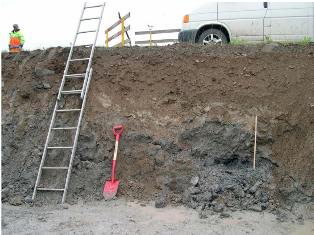
Figure 2-3. Photograph of artificial-fill profile in a trench (Hedenström and Sohlenius 2008).
