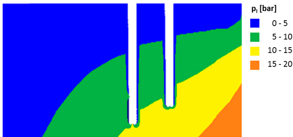
Figure 3-23. The average water pressures in the model about 3 months after installation of the bentonite.
