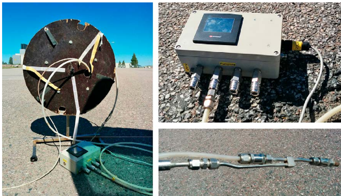
Figure 2-4. The equipment used for gas-lift pumping. On the left, the tubing lowered in the standpipe (the more narrow tube for sample water and the wider for gas) on a bobbin to simplify the lowering. To the upper right the control unit for the pumping/gas supply and lower right the end of the gas-lift pump.
