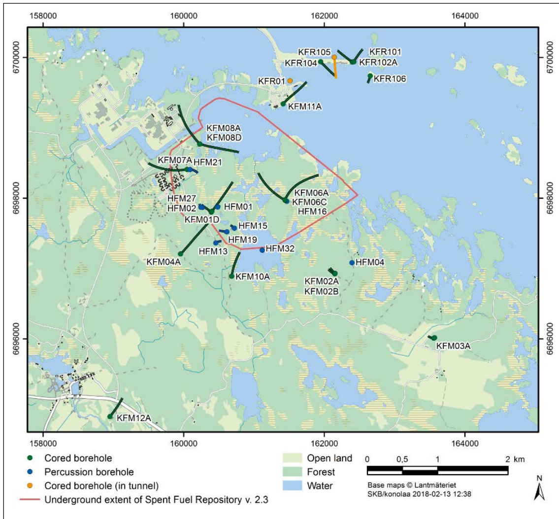
Figure 1-1. General overview of the Forsmark area and the boreholes included in the hydrochemical monitoring program for groundwater. The (telescopic) cored boreholes and the percussion boreholes within the monitoring program are marked with green and blue filled circles, respectively.
