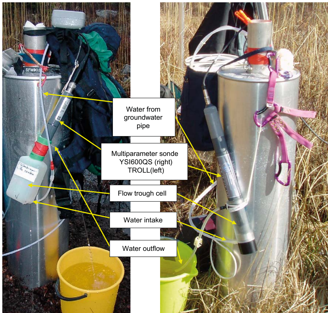
Figure 2-2. The multi parameter sonde used in 2015, Troll9500, to the right and the sonde used until April 2013, YSI 600 QS, to the left for comparison of set-up.
