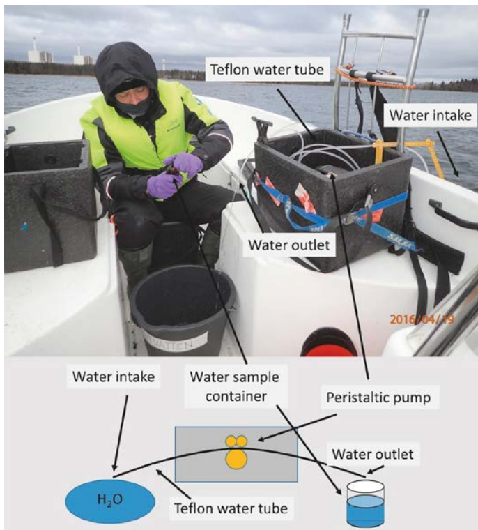
Figure 3-3. Winter sampling of surface water using the peristaltic pump system (PPS). A schematic presentation of the PPS is shown below the photo. Photo from the sampling at PFM00062.
