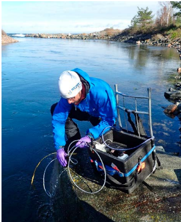
Figure 3-5. Sampling in the cooling water outlet (PFM102269).
