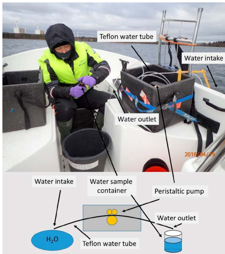
Figure 3-2. Winter sampling of surface water using the peristaltic pump system (PPS). A schematic presentation of the PPS is shown below the photo. Photo from the sampling at PFM00062.
