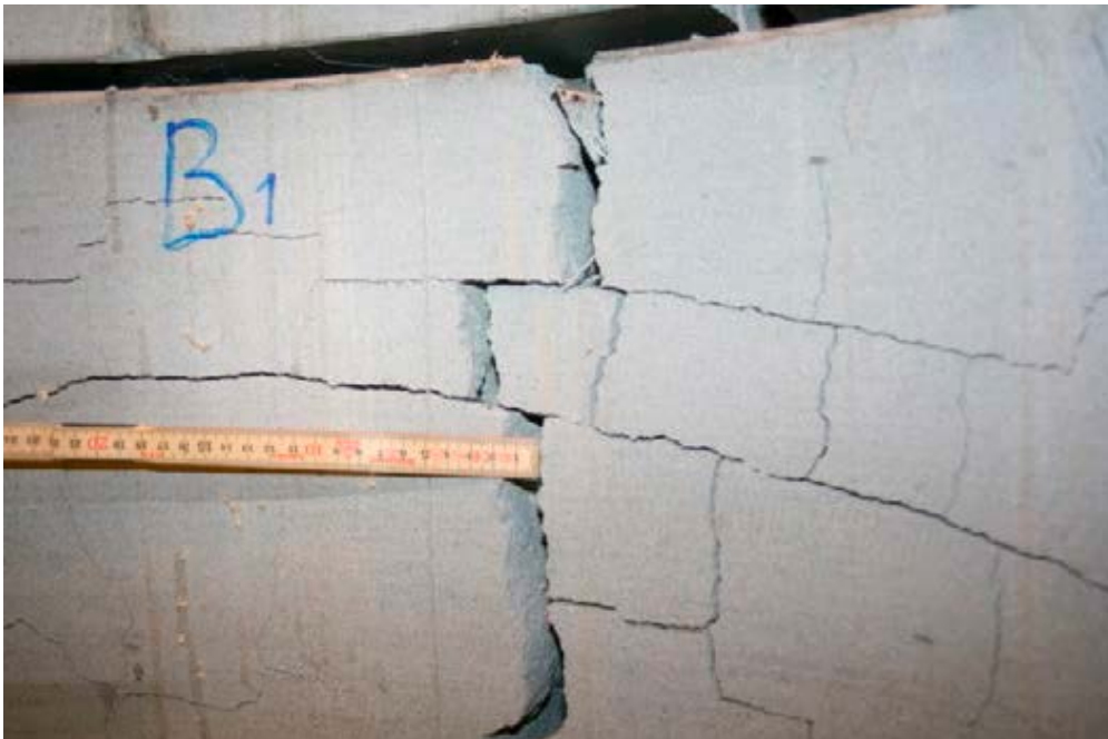
Figure 4-20. Cracking on the inside diameter of a buffer ring used in a heater test in Johannesson et al. (2014).
