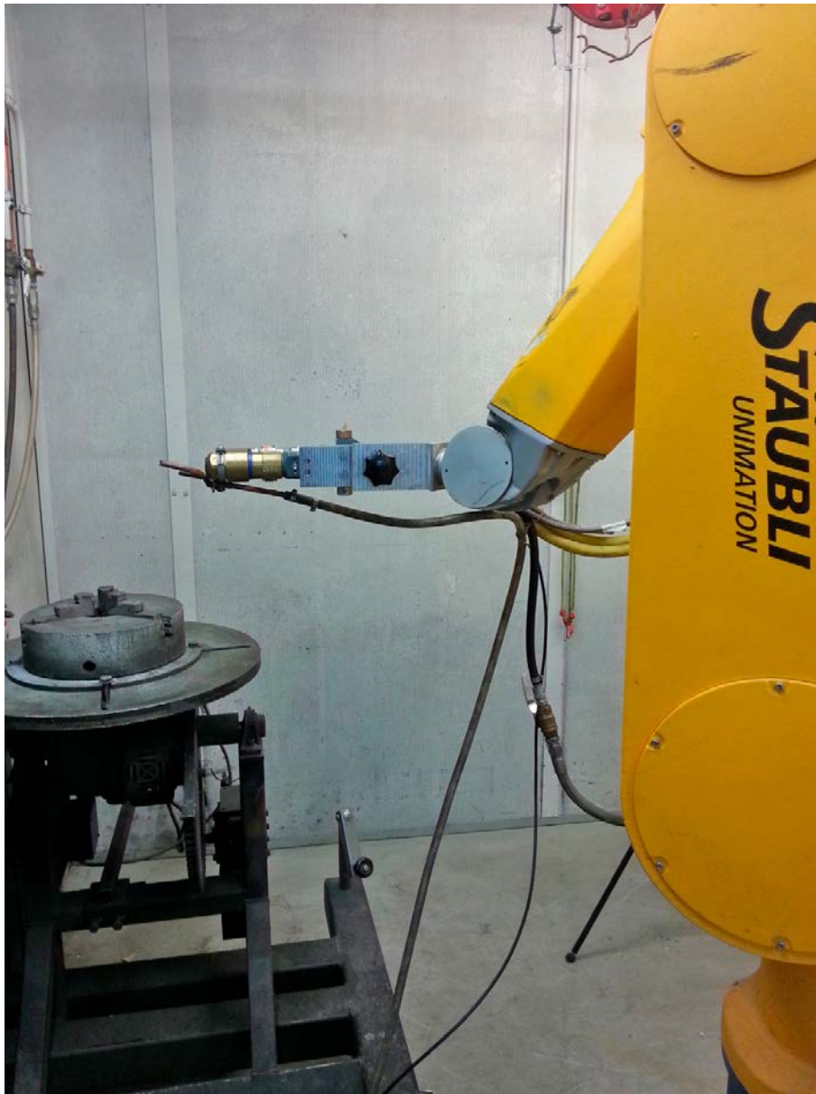
Figure 5-2. Robot with thermal spray gun used to coat the samples.
