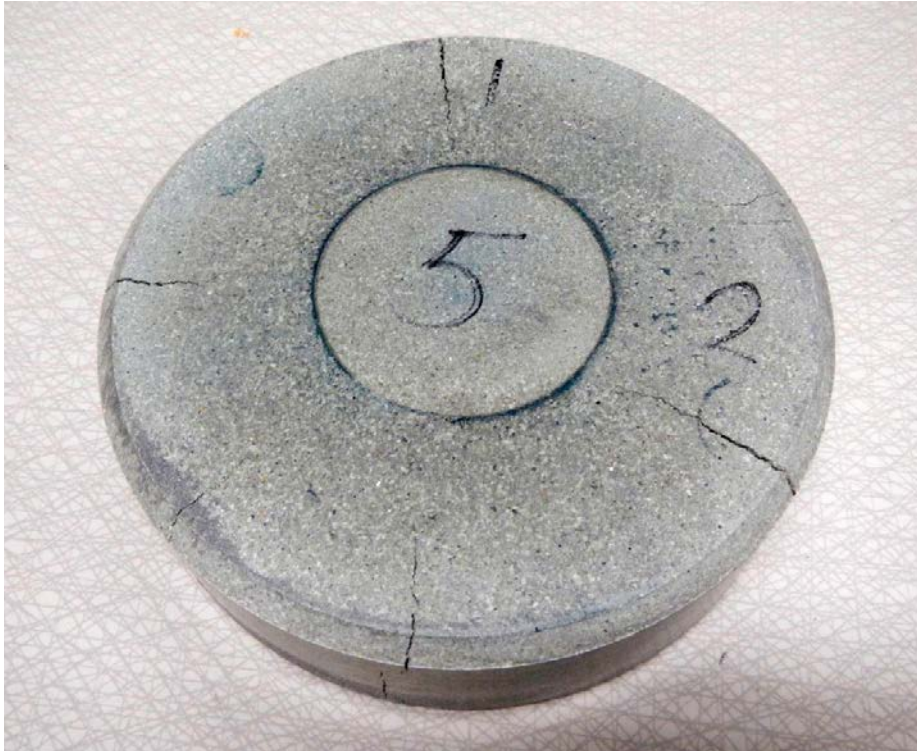
Figure 3-4. Photo showing cracks. The block has been taken out of the climate chamber after 16 days.
