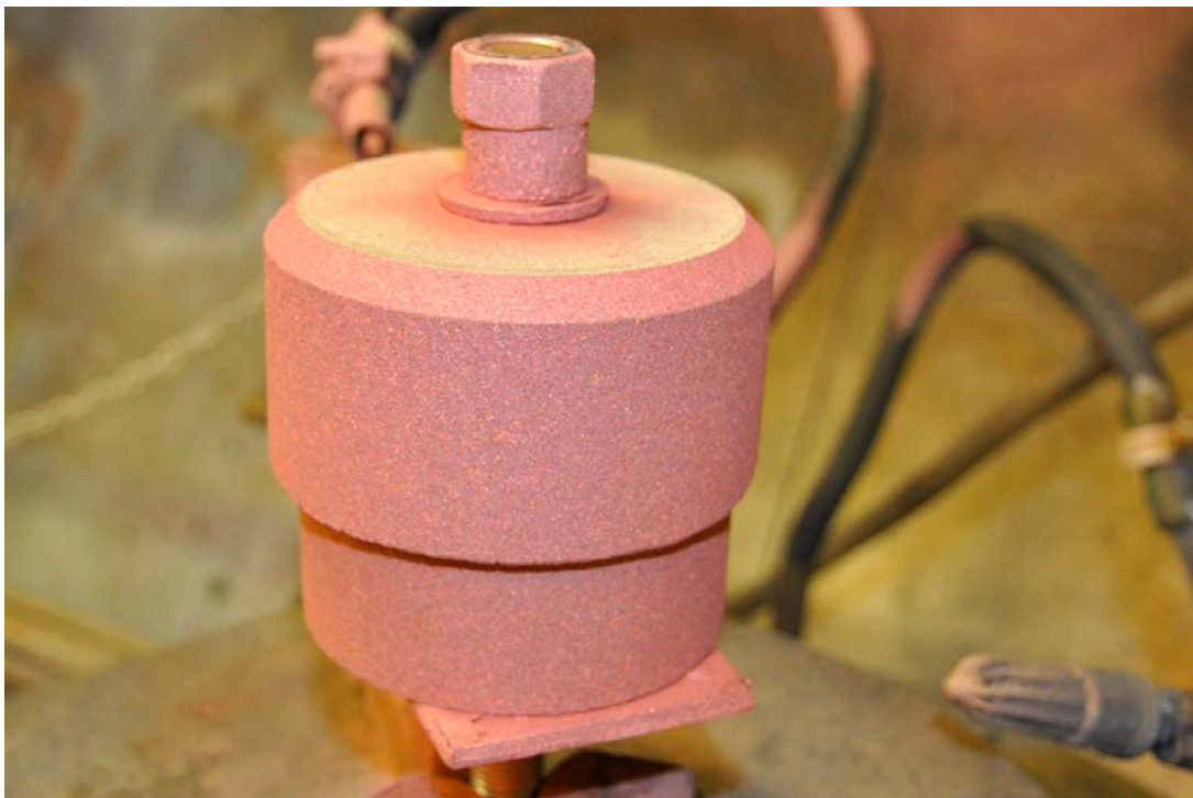
Figure 5-1. A small scale bentonite block coated with copper.
