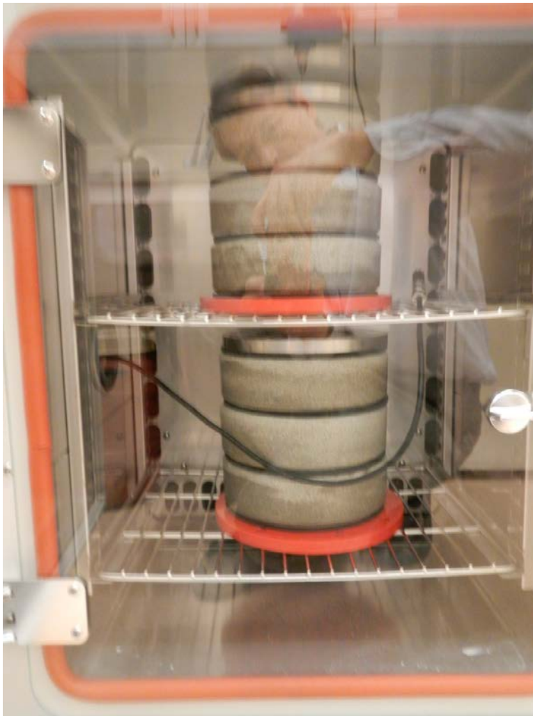
Figure 3-2. Photo showing the blocks after emplacement in the climate chamber.
