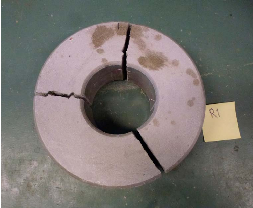
A1-12. Block R1 from above (direction 0° upwards). Several visible cracks.
