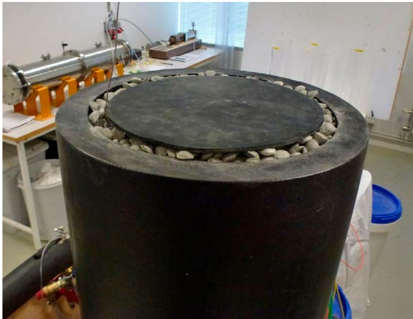
A1-6. The test setup with the rubber sheet on top and thermocouples C4 and T11 in place.
