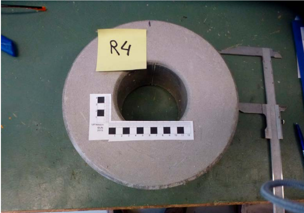
A1-8. Block R4 removed from the test (direction 0^\circ upwards). No visible cracks.
