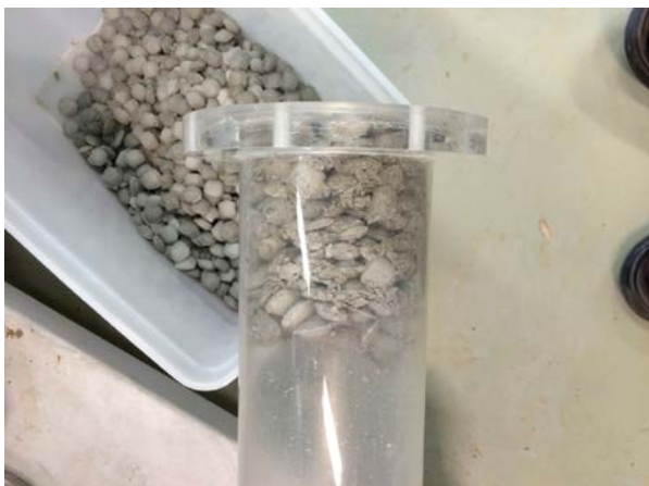
Figure 3-4. The pellets close to the air inlet at the dismantling of the 24 h test.
