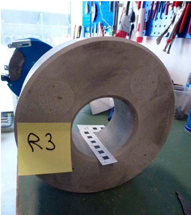
A1-9. Block R3 from below. A small crack is shown on the inside of the block.
