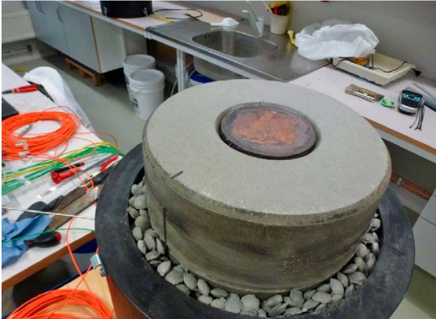
A1-5. Block R4 mounted and the outer slot filled with pellets. Thermocouples T2 and T10 with the heater are visible.
