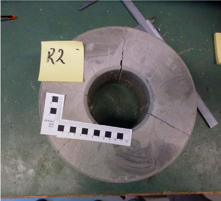
AI-10. Block R2 from below (direction 0° upwards). Several visible cracks.
