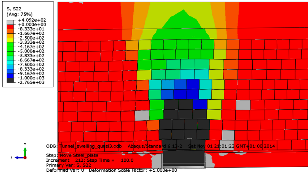
Figure 3-10. Vertical stress (kPa) after 10 cm displacement. Blocks with higher stress than 1 MPa are painted black.
