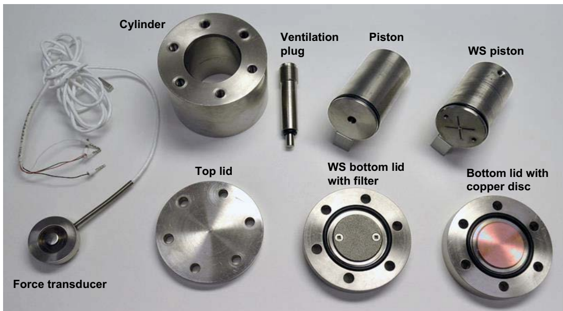
Figure 2-1. View of all parts included in a test cell. All parts in contact with the bentonites were made of titanium. See text for details. WS = water saturation.
