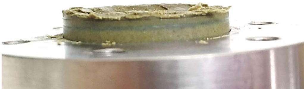
Figure 3-3. Profile view of the clay core in TC49 during sampling after 33 days. The dark line indicates the border between the two clay cores.
