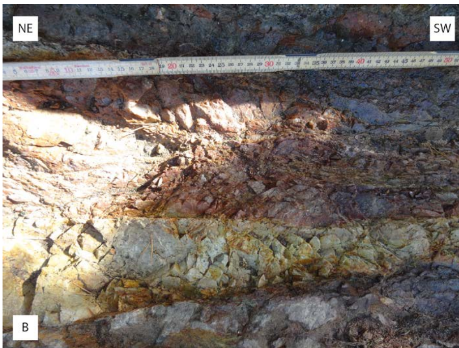
Figure 3-9. b) Cataclasite in the core of the Äspö shear zone. The cataclasite consists of a c. 30 cm wide brittle shear zone that has undergone extreme alteration. Location: PAS000633 (X6368009, Y1551230).
