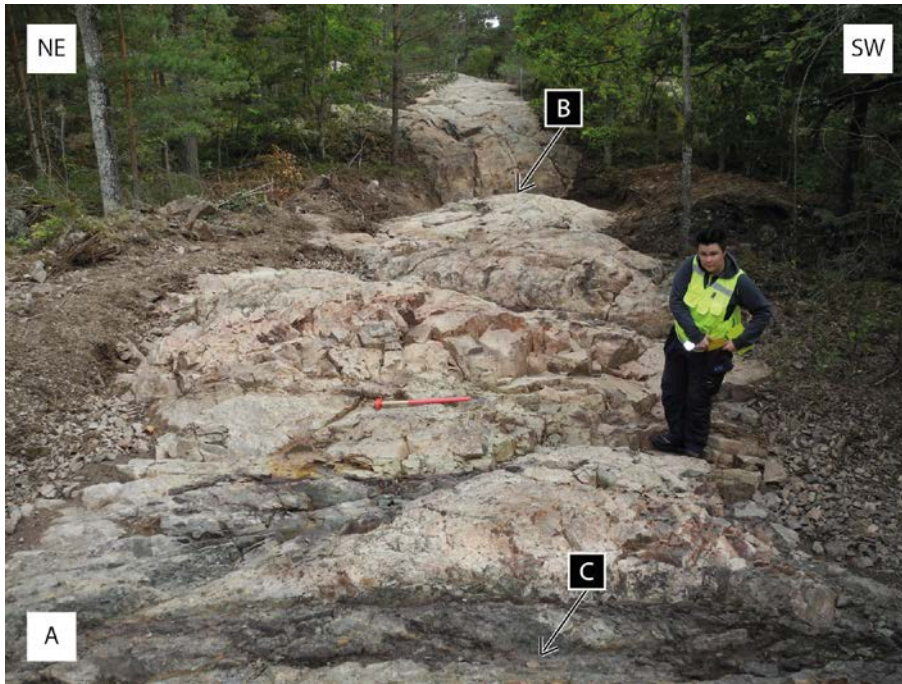
Figure 3-9. a) Cleaned trench across the central part of the Äspö shear zone. Chemical alteration can be observed across a c. 20 m wide zone (across the entire photography) and gives the rock a light grey to pink appearance.
