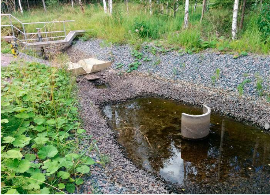
Figure 4-1. Dry flume and zero discharge at gauging station PFM005764 on August 5, 2016.
