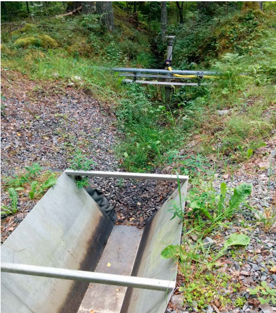
Figure 4-2. Dry flume and zero discharge at gauging station PFM002668 on August 5, 2016.
