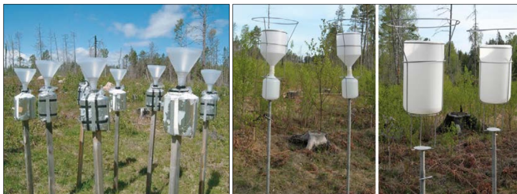
Figure 6-7. In 2003, the sampling location for precipitation was moved from PFM002457 to PFM002564 due to suspected dust contamination from a gravelled road with increasing traffic. The first samplers that were used for collecting the precipitation were very simple (to the left) and they were changed for more adequate ones in 2007 (middle and right). Different types were used for collecting rain (middle) and snow (right). No sampling of precipitation for hydrochemical analyses has been performed since 2012.
