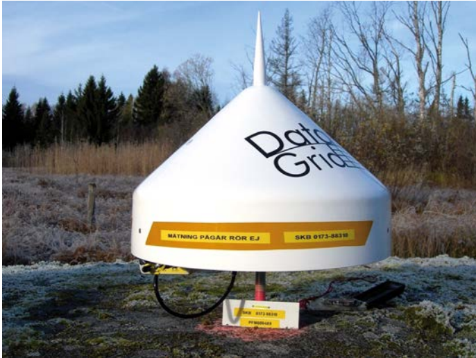
Figure 4-9. Sampling station at Forsmark with a choke ring antenna and GPS receiver mounted to the lower left. All stations are attached to a short steel rod anchored to the rock for good mechanical and thermal stability. The selection of the GPS sampling sites at Forsmark was based on geological assessments as well as on considerations about sky visibility and nearby natural or man-made reflectors (Figure 3-1 in Gustafson and Ljungberg 2010).
