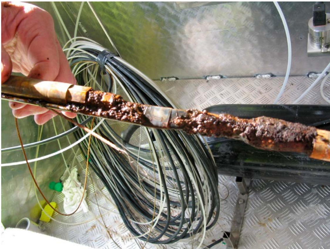
Figure 4-24. Corroded monitoring equipment in drill hole KFM08B in 2012. This particular component had been installed in the borehole, after service, only two months earlier.
