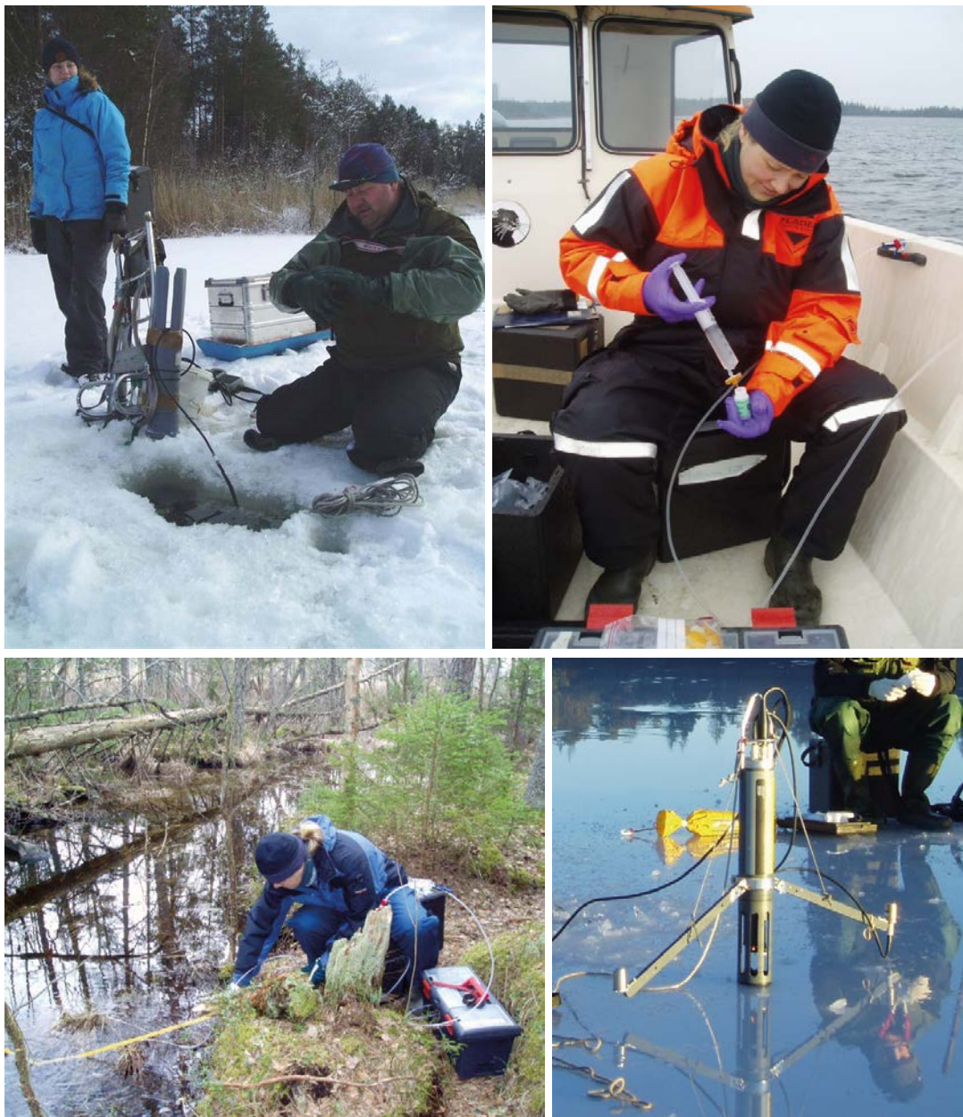
Figure 6-2. Field probe measurements in Lake Norra Bassängen from the ice during winter (upper left). Sea water samples are filtered directly in the field (upper right). Sampling of the stream at the outlet of Lake Eckarfjärden is performed using of a peristaltic pump at a depth of c 0.1 m. The multi-parameter probe YSI 6600 EDS was used for field measurements until 2013 when it was replaced with InSitu Troll9500.
