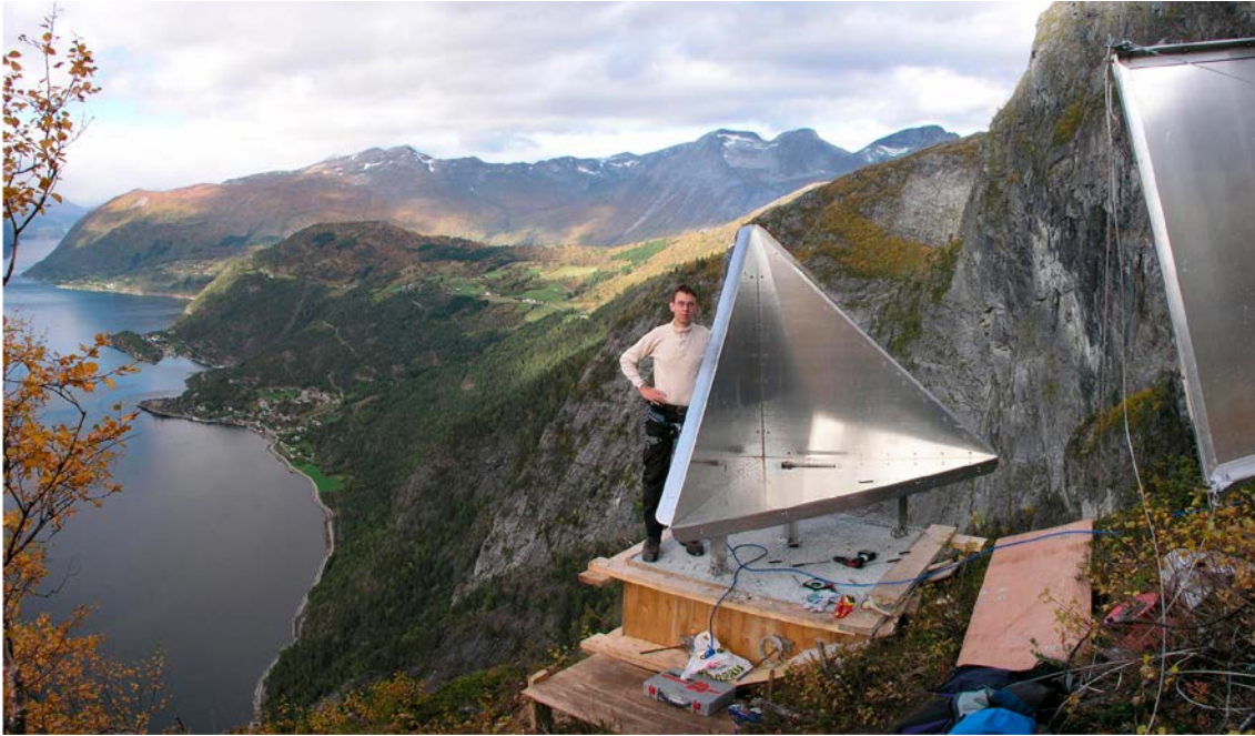
Figure 8-1. Artificial PS corner reflector installed near Tafford, in Norway. The reflector is constructed of 10 mm thick aluminium. Figure from Dehls (2006, Figure 4-1).
