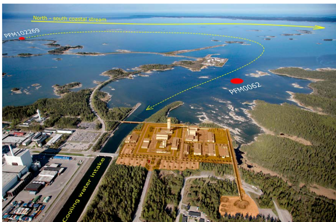
Figure 8-3. Photo montage including planned future surface facilities related to the spent fuel repository and the present single sea-water sampling location in Asphällsfjärden (PFM000062) as well as a suggested sampling location at the cooling-water outlet in Lake Biotestsjön (PFM102269). The first location is significantly influenced from the cooling-water intake to the nuclear power plant. The sampling location at the cooling-water outlet in Lake Biotestsjön (PFM102269) is presently used only for checks of tritium emissions and it is recommended to introduce the same analytical protocol as for the other sea-water locations at that location. Along the coast, there is a predominating north-south coastal stream, and the dashed line marks the likely circulation of the cooling water from the nuclear power plant.
