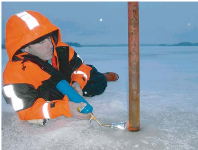
Figure 6-20. Defrosting ice inside a steel monitoring well located in a lake, using an LPG burner.
