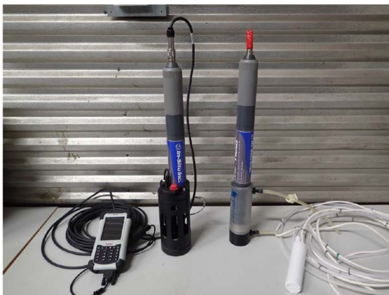
Figure 6-22. The probes used for measurements in surface water (left) and near surface groundwater (right). The rightmost probe is equipped with a flow-through cell and a submersible pump (white) for measurements in monitoring wells.
