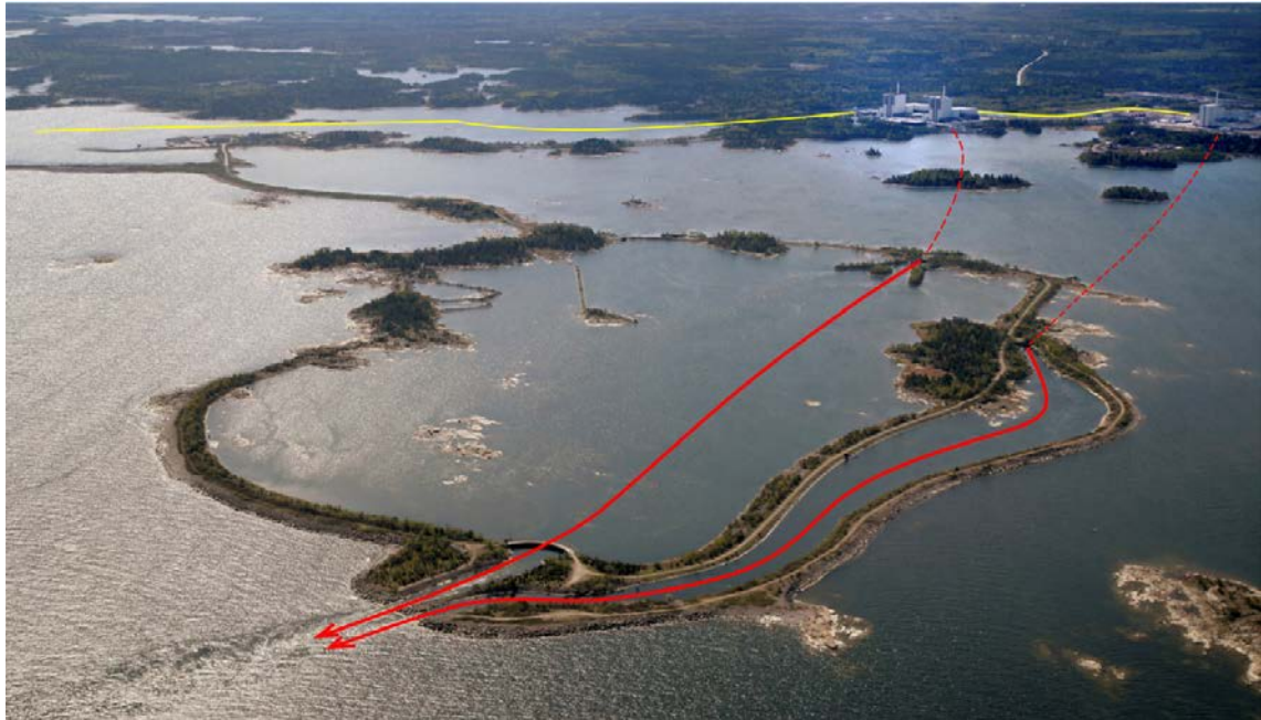
Figure 6-6. Tritium is sampled near the outlet of Lake Biotestsjön that receives cooling water from the nuclear power plants. Cool sea water reaches the reactors along the yellow line via the inlet canal. Heated cooling water is led to the lake via tunnels below the sea floor according to the schematic dashed red lines. Cooling water from reactor 1 and 2, and 3, respectively, mix when the separate currents reach the Baltic Sea (solid red lines).
