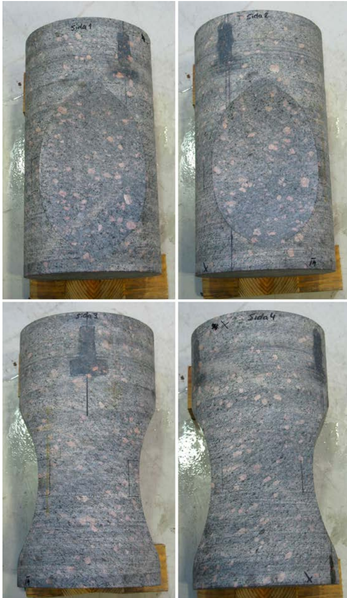
Figure 2-4. Specimen KS0041B02. Sides 1–4. The surface has been slightly grinded in the darker areas on the top of the specimen for subsequent strain gauge installation.
