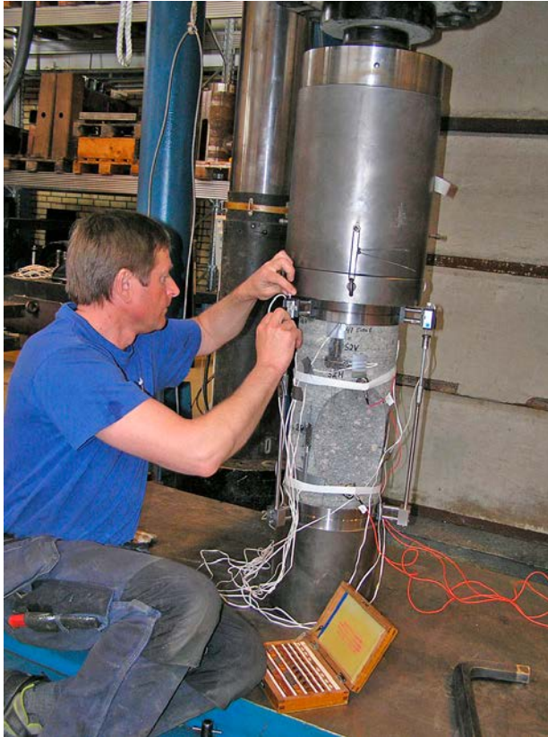
Figure 2-10. Calibration check of the LVDTs by means of gauge blocks (Johansson gauge) prior to the test of KS0041B02.
