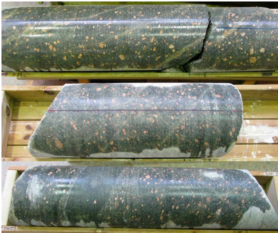
Figure 2-1. Specimens after they arrived to SP. Upper picture: KS0037B02; Middle picture: KS0041B02; Lower picture: KS0044B02. The surfaces of the cores were moistured in order to better reveal the rock texture.
