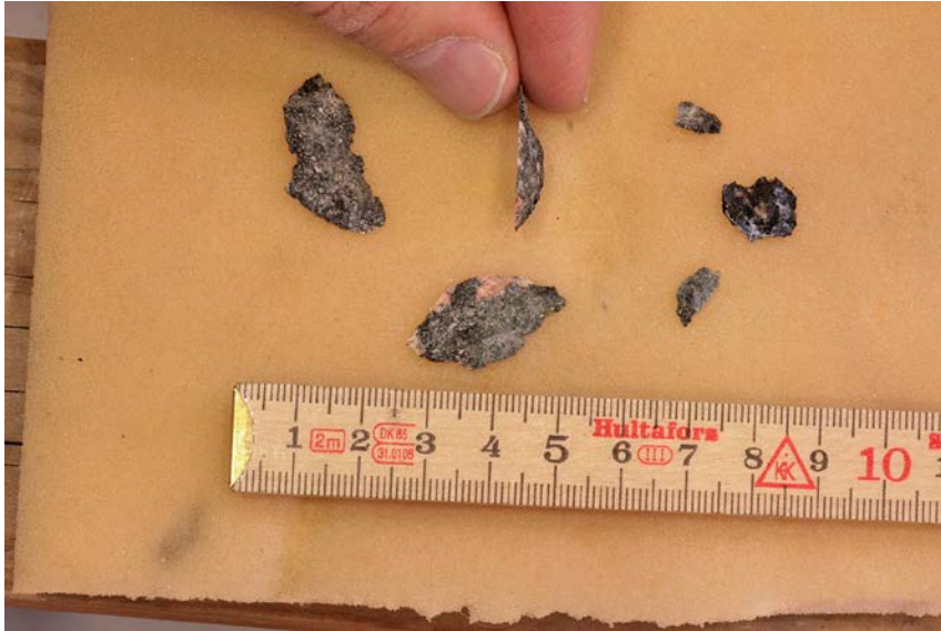
Figure 5-8. Chips that has fallen off specimen KS0044B02. The pieces are up to 25–28 mm, thickness/depth about 5 mm.
