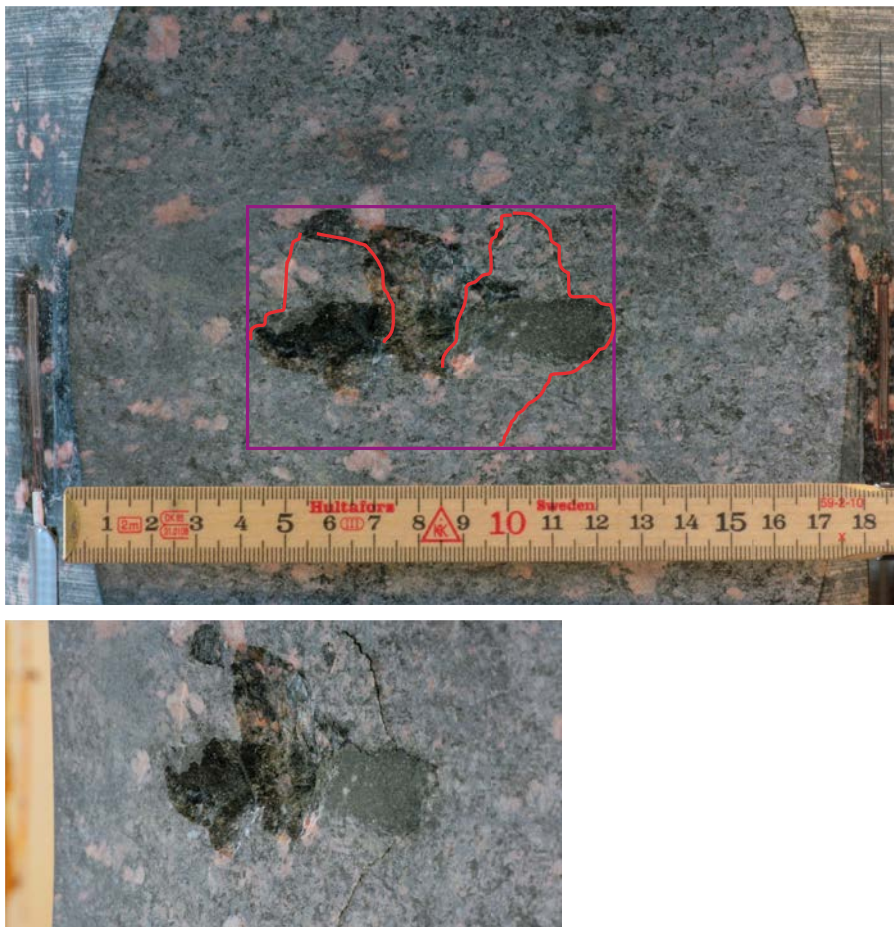
Figure 5-7. Specimen KS0044B02 side 1. Spalling in the centre of the notch ( 85 \times 45 mm) Upper picture: The red lines show the crack pattern of fully developed cracks; Lower picture: As above, but seen from the side. Chips of the rock material have fallen off the surface. Fractures around the long mafitic xenolith are visible.
