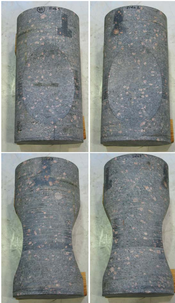
Figure 2-5. Specimen KS0044B02. Sides 1–4. The surface has been slightly grinded in the darker areas on the top of the specimen for subsequent strain gauge installation. A long mafitic xenoliths in the horizontal direction is seen at the centre on the notch on side 1 (upper left figure).
