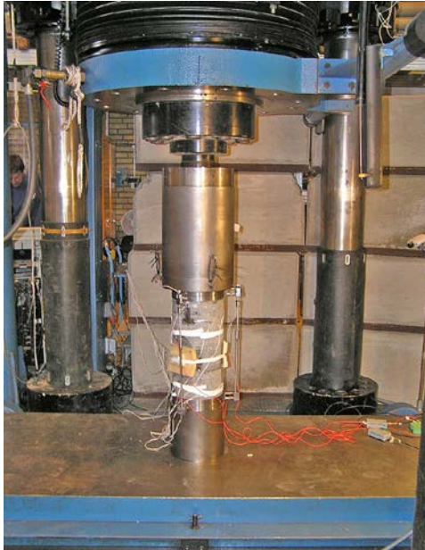
Figure 2-6. Specimen KS0044B02 placed in the load frame right before testing. The concrete blocks sealing off towards the control area are seen in the background.
