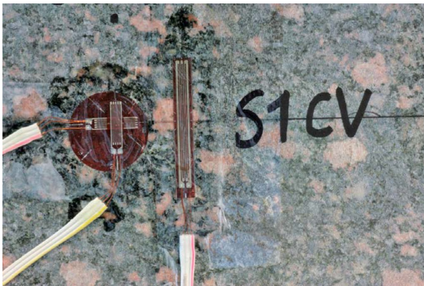
Figure 4-9. Centre of the notch at side 1 of specimen KS0041B02 after testing. Some cracks are visible.
