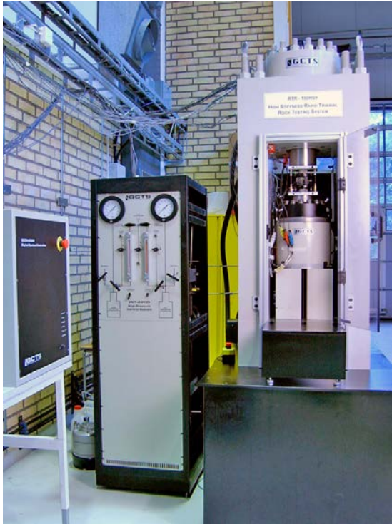
Figure A-1. Rock testing system. From left: Digital controller unit, pressure cabinet (used for triaxial tests) and load frame. The PC with the test software (not shown in the picture) is placed on the left hand side of the controller unit.
