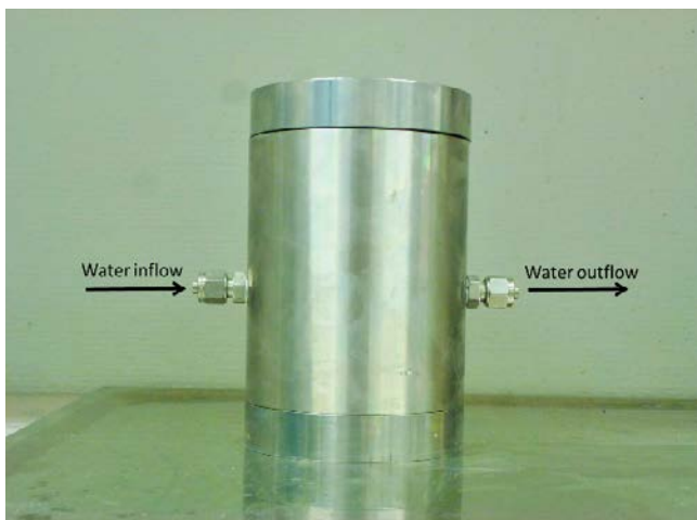
Figure 10-5. Photo of the device used for the piping (erosion) tests with D = 60 mm and H = 120 mm. The arrows show the water in- and out-flow.
