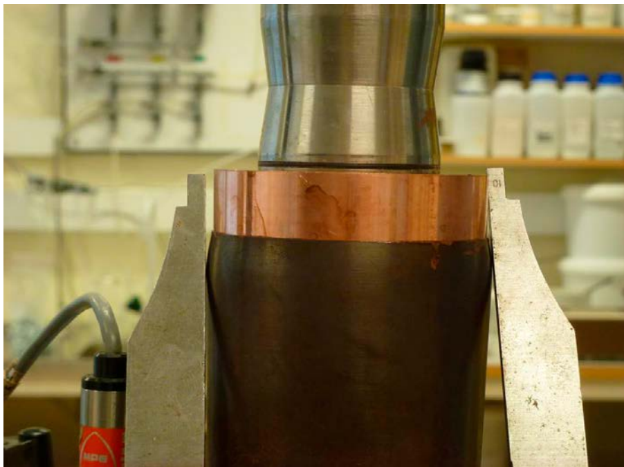
Figure 6-4. Copper expander after compression with 100 kN.
