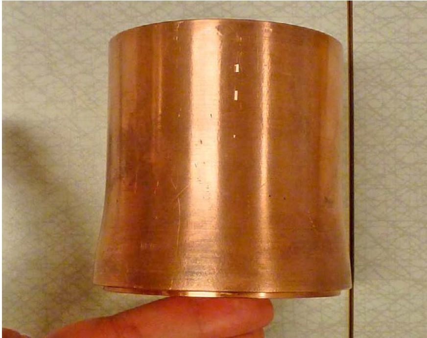
Figure 6-9. Photo showing the copper expander after compression. The lower part has been clearly expanded.
