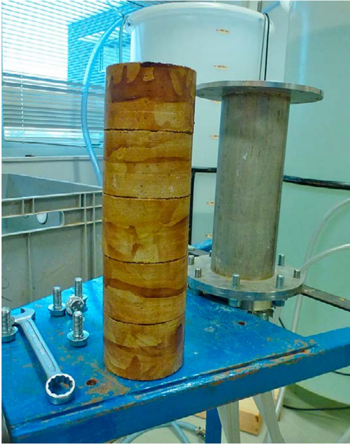
Figure 7-1. Photo of blocks ready for installation. The blocks on the photo are coated with shellac.
