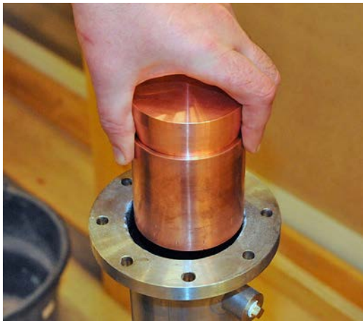
Figure 8-4. Installation of a copper expander in the simulated borehole.
