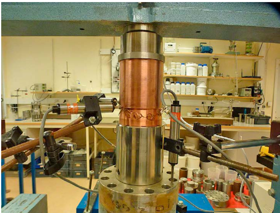
Figure 6-6. Photo showing the test setup just before starting the compression. Note that the conical part is at the bottom. This part is also lubricated with copper paste in order to decrease the friction additionally.
