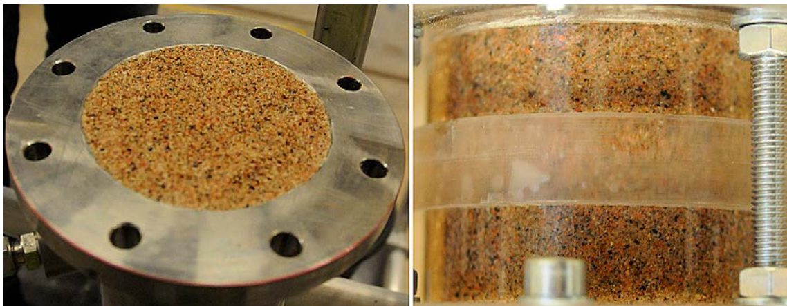
Figure 8-3. Left: The top of the uppermost sand section. Right: Close-up of the lower sand filled section. The photo is taken through one of the Plexiglas sections.
