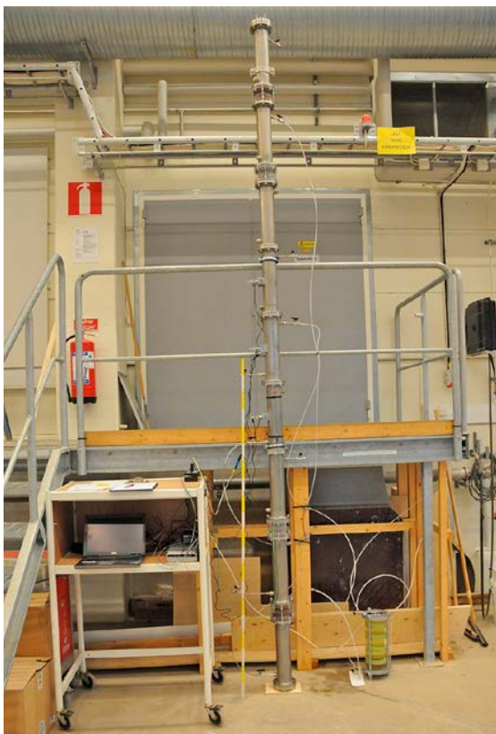
Figure 8-8. Overview of the test setup after having finished the installation. The vessel on the floor to the right contains the pressurized water.
