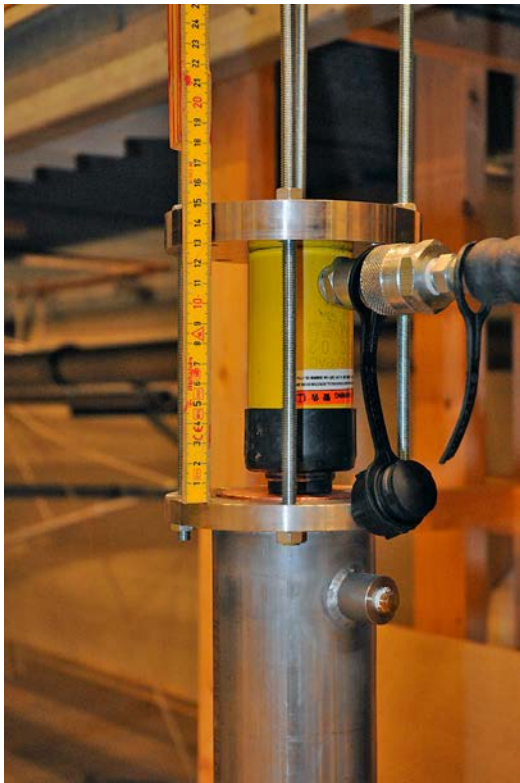
Figure 8-5. A hydraulic piston was used to compress the copper expander.
