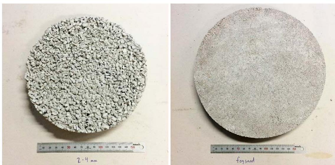
Figure 5-1. Left: Concrete using Ballast 2–4 mm Right: Concrete using Fogsand 0–2 mm.
