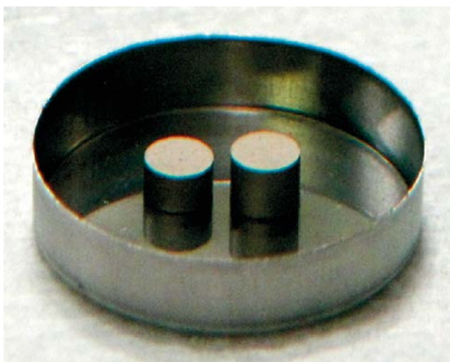
Figure 3-4. (Pu,Zr)N pellets fabricated by KTH in JAEA labs.
