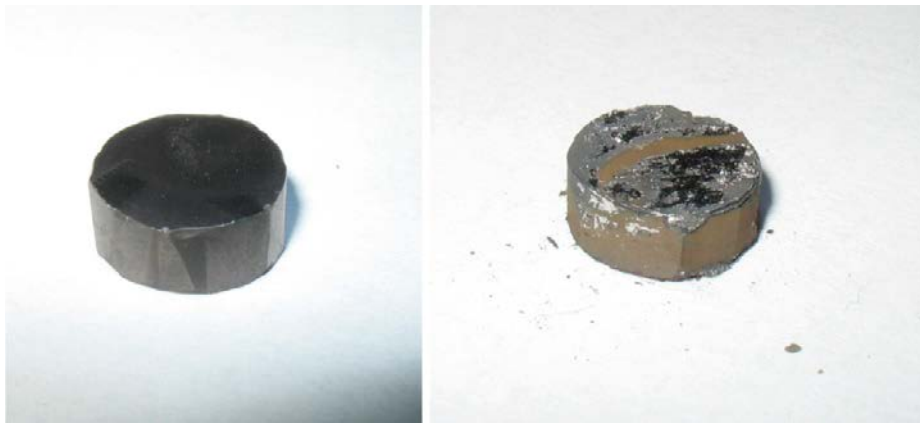
Figure 3-13. UN pellet subjected to thermal shock, before (left) and after (right) the experiment.
