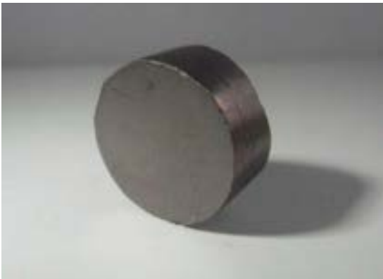
Figure 3-2. Spark plasma sintered UN pellet.
