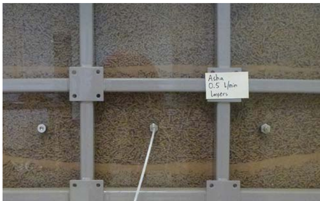
Figure 4-8. Photos showing the wetting pattern at time for termination. Upper: AL_0.5_0 (Asha, 0.5 l/min and sieved pellets) Lower: AL_0.5_L (Asha, 0.5 l/min, fines in layers)
