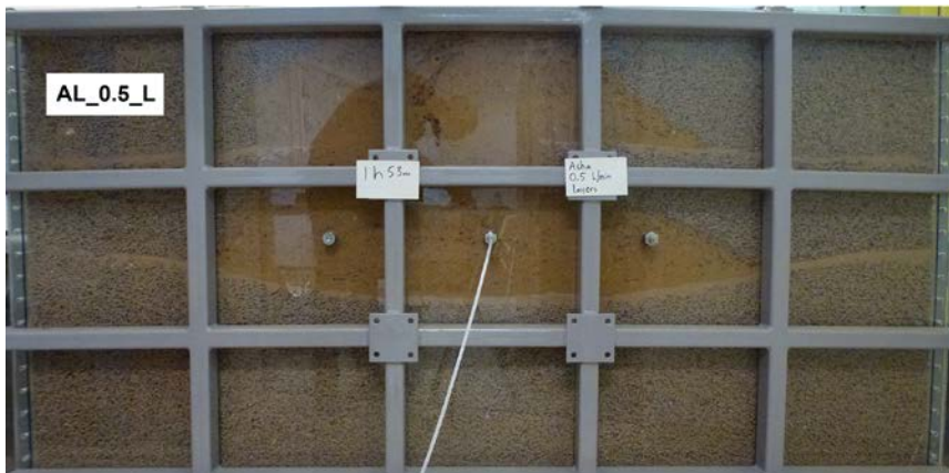
Figure 4-8. Photos showing the wetting pattern at time for termination. Upper: AL_0.5_0 (Asha, 0.5 l/min and sieved pellets) Lower: AL_0.5_L (Asha, 0.5 l/min, fines in layers)
