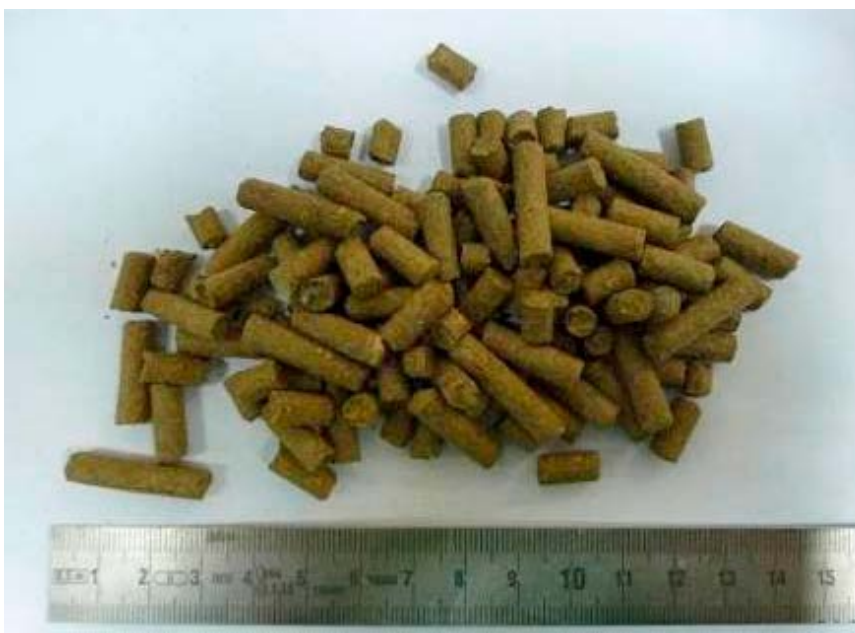
Figure 3-2. Asha extruded 6 mm pellets used in the Tube tests.
