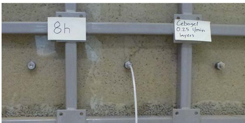
Figure 4-23. Photos showing close-ups of the test performed with layers, CL_0.25_L (Cebogel, 0.25 l/min, fines in layers). Upper: After installation Lower: At termination.
