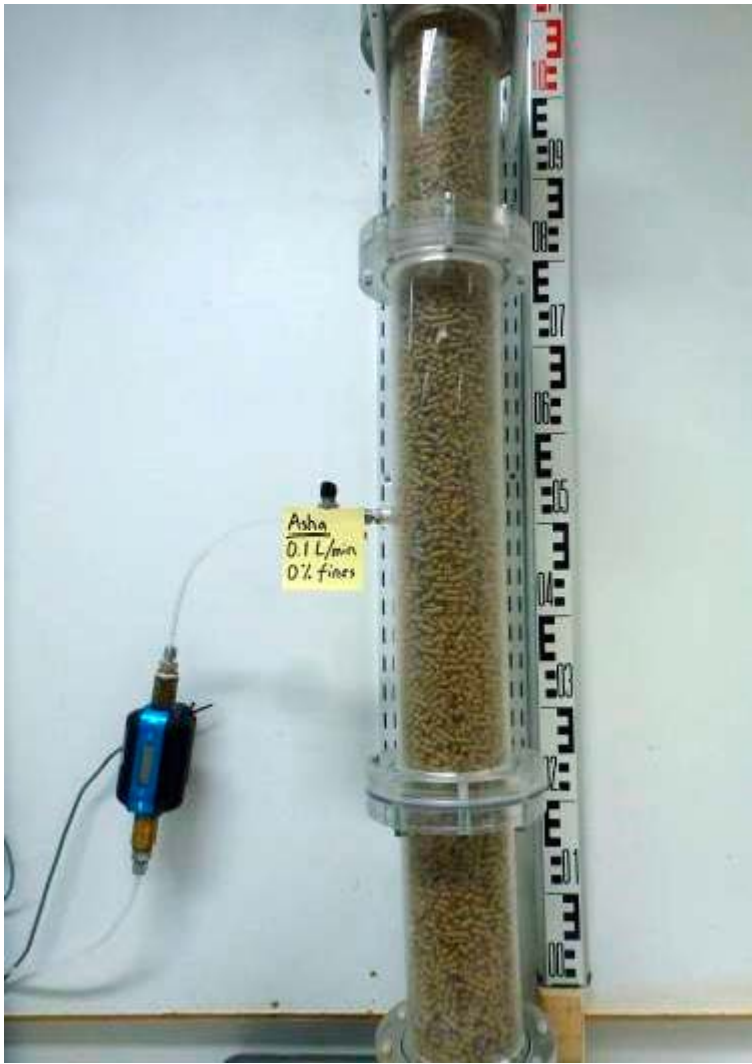
Figure 3-1. The “Tube test” equipment used for studying the influence of fines in the pellet filling.
