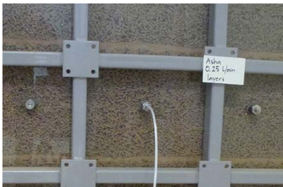
Figure 4-5. Photos showing the wetting pattern at time for termination. Upper: AL_0.25_0 (Asha, 0.25 l/min and sieved pellets) Lower: AL_0.25_L (Asha, 0.25 l/min, fines in layers)
