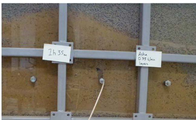
Figure 4-12. Photos showing close-ups of the test performed with layers, AL_0.75_L (Asha, 0.75 l/min, fines in layers). Upper: After installation Lower: At termination.
