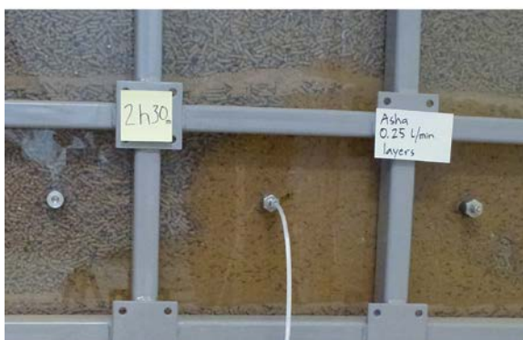
Figure 4-6. Photos showing close-ups of the test performed with layers, AL_0.25_L (Asha, 0.1 l/min, fines in layers). Upper: After installation Lower: At termination.
