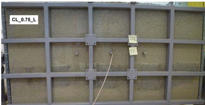
Figure 4-22. Photos showing the wetting pattern at time for termination. Upper: CL_0.25_L (Cebogel, 0.25 l/min with layers) Lower: CL_0.75_L (Cebogel, 0.75 l/min with layers).
