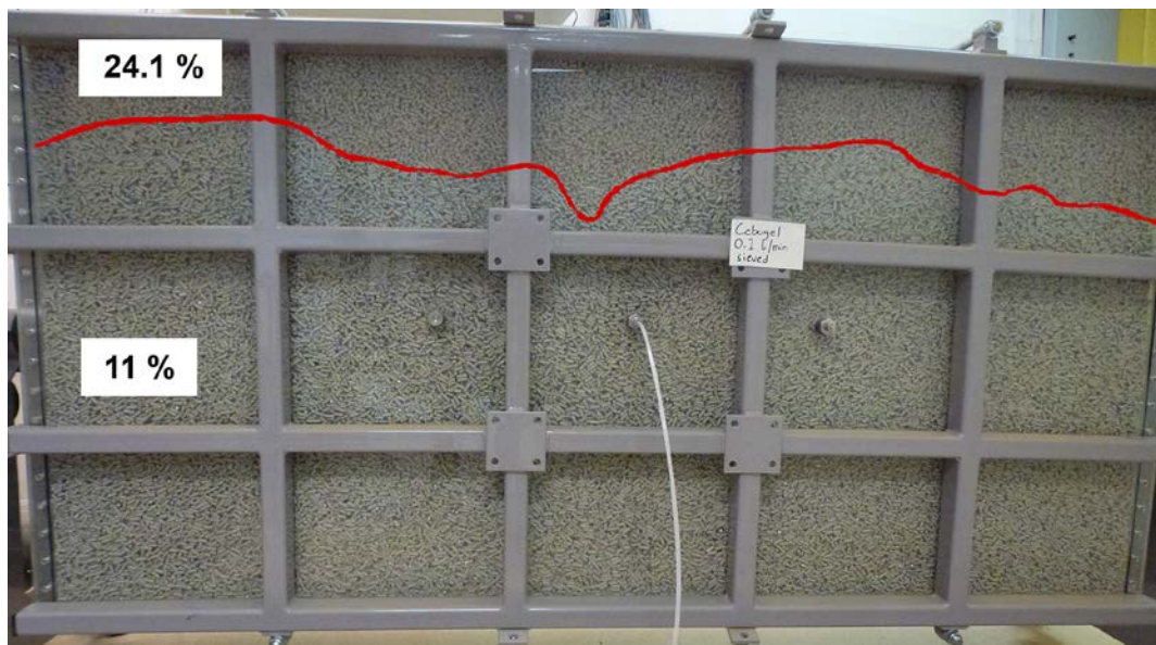
Figure 4-16. Photos showing a photo of the Test CL_0.1_mix after installation of pellets from two different batches. There was a visually very clear difference between the two batches.
