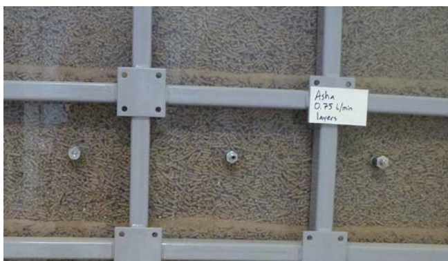
Figure 4-11. Photos showing the wetting pattern at time for termination. Upper: AL_0.75_0 (Asha, 0.75 l/min and sieved pellets) Lower: AL_0.75_L (Asha, 0.75 l/min, fines in layers)
