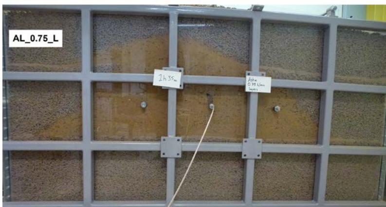
Figure 4-11. Photos showing the wetting pattern at time for termination. Upper: AL_0.75_0 (Asha, 0.75 l/min and sieved pellets) Lower: AL_0.75_L (Asha, 0.75 l/min, fines in layers)
