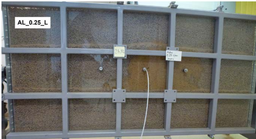
Figure 4-5. Photos showing the wetting pattern at time for termination. Upper: AL_0.25_0 (Asha, 0.25 l/min and sieved pellets) Lower: AL_0.25_L (Asha, 0.25 l/min, fines in layers)
