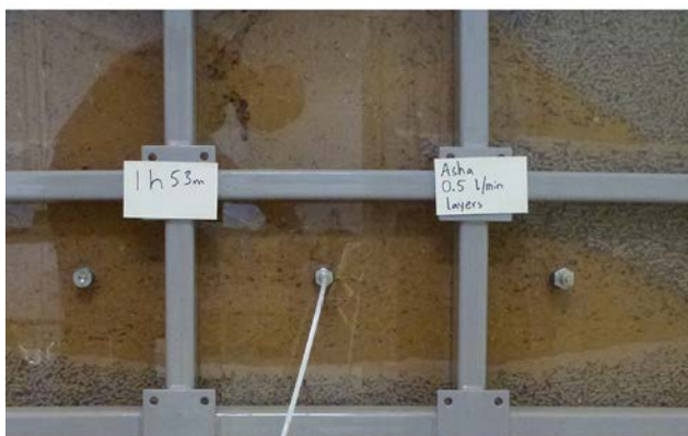
Figure 4-9. Photos showing close-ups of the test performed with layers, AL_0.5_L (Asha, 0.5 l/min, fines in layers). Upper: After installation Lower: At termination.
