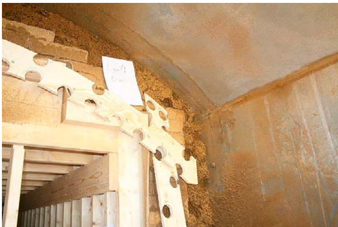
Figure 4-9. Photo showing the templates used for sampling of the pellet filled slot.
