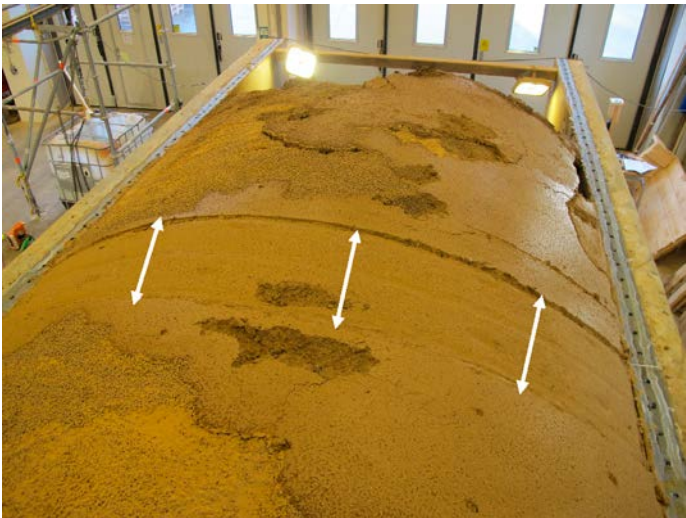
Figure 4-43. Photo showing the pellet ceiling after having removed the steel roof in Test 5. Location of geotextile indicated with white arrows. Inflow port is on right side)
