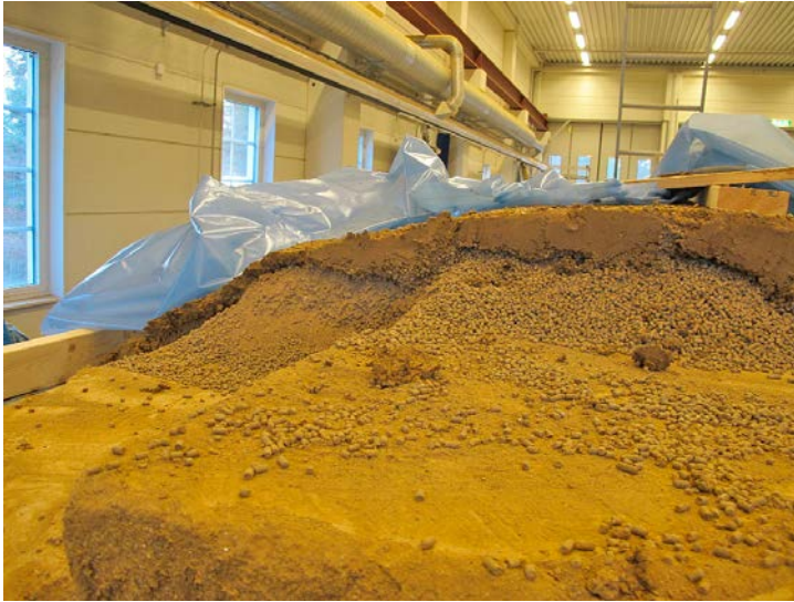
Figure 4-44. Photo showing a cross section of the pellet filling at the top of the tunnel in Test 5. The inflowing water has followed the geotextile up over the top and down on the other side of the tunnel (inflow side to the left in the photo).
