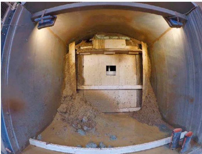
Figure 4-16. Photo showing Test 2 after 135 hours test duration. A large water breakthrough has occurred at the front.
