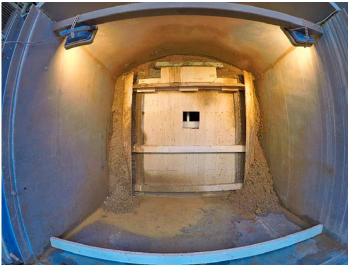
Figure 4-15. Photo showing the backfill front in Test 2 after approximately 120 hours test duration.
