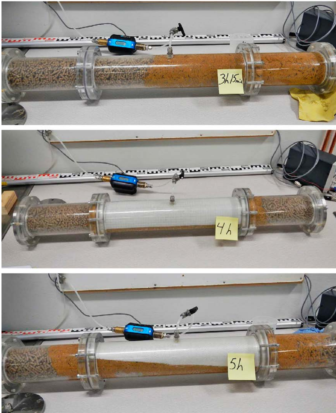
Figure 3-1. Photo of the three tests. Upper: Reference test Middle: Test performed with geotextile TG660 Lower: Test performed with geotextile TG1000.
