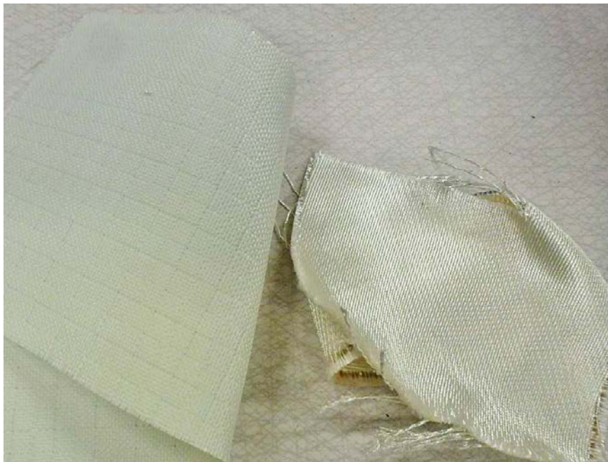
Figure 2-1. Samples of glass fiber based geotextiles. The one to the right was judged to be most feasible as water distributor in the steel tunnel tests.
