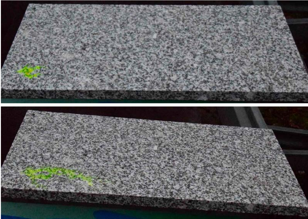
Figure A-33. Granite slab with moving film generated by slight drizzle. First frame after emplacement of dye drop. Second frame 20 minutes later. Slope of slab is about 5 cm/m.
