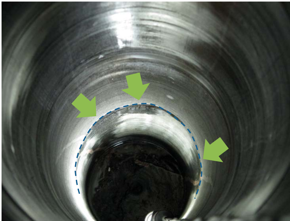
Figure 7-33. Location of inflows along fracture at 2.9 m in KO0017G01. See also the pegmatite vein that may conduct water.
