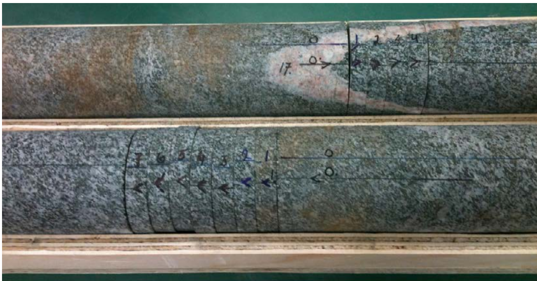
Figure 7-24. Photo: Diorite-pegmatite (upper core, KO0017G01) and diorite (lower core, KO0018G01).
