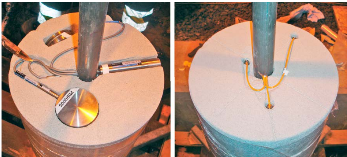
Figure 7-10. Instrumentation of blocks; left: block with pressures sensors; right: block with RH sensors.
