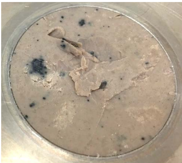
Figure 3-4. Black spots observed during sampling of test cell with GMZ bentonite.
