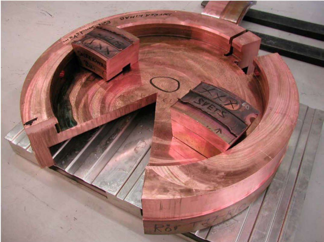
Figure 2-1. Welded lid and ring from which specimens were extracted.
