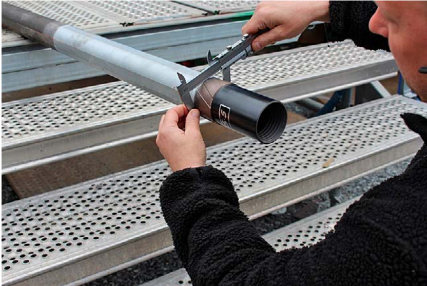
Figure 5-6. The Hexgon core barrel used for conventional drilling in N-size.
